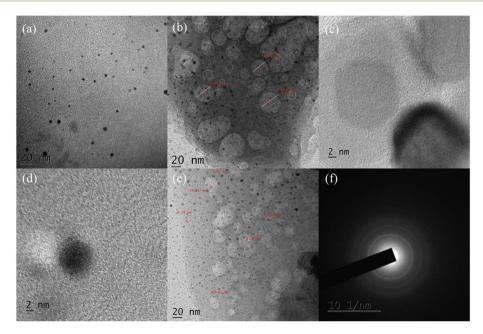
Fig. 5 (a and d) HRTEM images of SPIONs, (b, c and e) morphological features of the SPION-AC nanocomposite, and (f) the SAED pattern of the synthesized SPION-AC nanocomposite.
