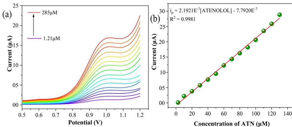
Fig. 11 (a) Voltammograms representing the DPV curves for ATN oxidation at the SPION-15%AC/GCE surface in BR buffer solution (pH 10) at a scan rate of  $0.05 \text{ V s}^{-1}$ , (b) calibration plot for the DPV curves under the same experimental conditions.
