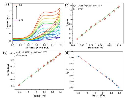
Fig. 9 (a) Superimposed cyclic voltammograms for the electrochemical detection of 80 µM ATN in BR buffer solution (pH 10) at varying scan rates between  $0.01\,\mathrm{V\,s^{-1}}$  to  $0.1\,\mathrm{V\,s^{-1}}$ , (b) a plot of scan rate versus ATN oxidation peak current, (c) a log-log plot of scan rate versus ATN oxidation peak current, and (d) linear plot of logarithm of scan rate versus peak potential.
