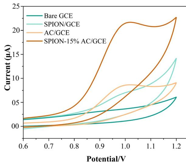
Fig. 8 Superimposed cyclic voltammograms for the electrochemical detection of 80  $\mu$ M ATN at 0.05 V s<sup>-1</sup> in BR buffer solution of pH 10 at the bare GCE, SPION/GCE, AC/GCE, and SPION-15%AC/GCE surfaces.
