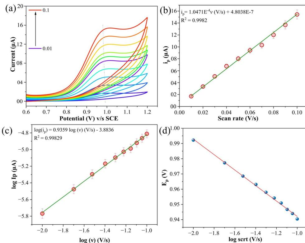
Fig. 9 (a) Superimposed cyclic voltammograms for the electrochemical detection of 80  $\mu\text{M}$  ATN in BR buffer solution (pH 10) at varying scan rates between 0.01  $\text{V s}^{-1}$  to 0.1  $\text{V s}^{-1}$ , (b) a plot of scan rate *versus* ATN oxidation peak current, (c) a log-log plot of scan rate *versus* ATN oxidation peak current, and (d) linear plot of logarithm of scan rate *versus* peak potential.
