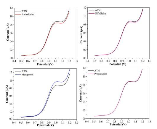
Fig. 12 Interference studies of SPION-15%AC/GCE for 80 μM ATN and 800 μM amlodipine besylate, nifedipine, metoprolol and propranolol.
