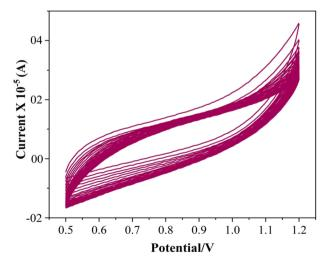
Fig. 13 Cyclic voltammogram of SPION-15%AC/GCE at the scan rate of 0.05 V s $^{-1}$  in 0.04 M BR buffer (pH 10), run continuously for 25 cycles.
