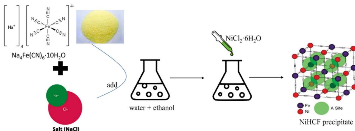
Fig. 7 Schematic of synthesis of nickel hexacyanoferrate.
