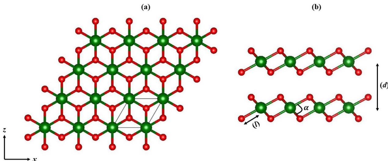
**Fig. 1** Optimized crystal structure of an  $XO_2$  bilayer with (a) top view and (b) side view. Green and red atoms represent X and O atoms, respectively.
