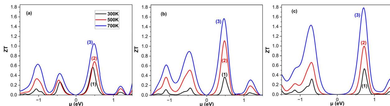
**Fig. 5** Figure of merit (ZT) of (a) NiO<sub>2</sub> (b) PdO<sub>2</sub> and (c) PtO<sub>2</sub> bilayers as a function of chemical potential at various temperatures.
