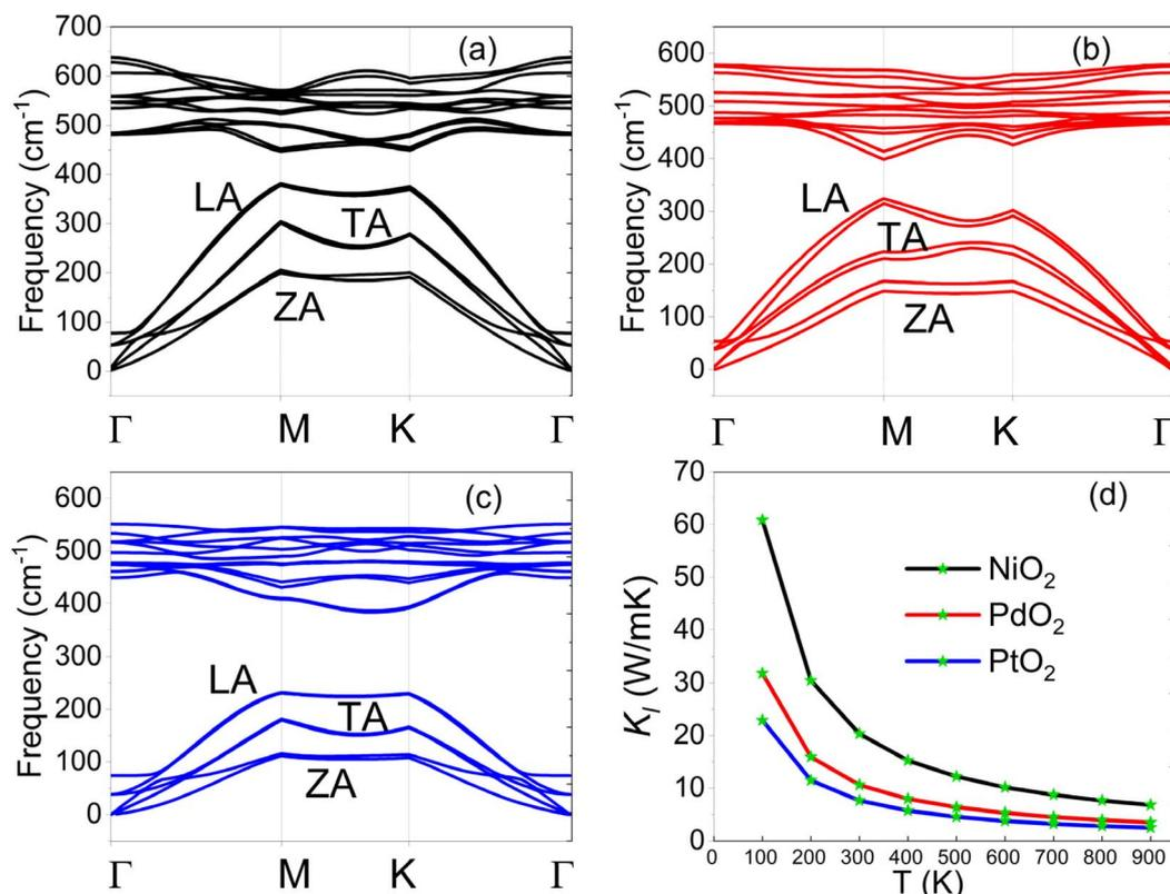
Fig. 3 Plots depicting phonon band structures (a–c) and lattice thermal conductivity (d) of XO<sub>2</sub> bilayers at various temperatures.
