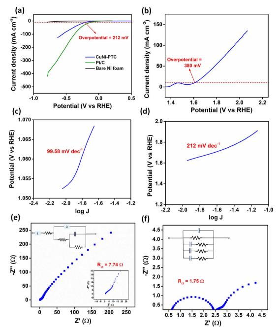
Fig. 7 (a and b) LSV curves, (c and d) Tafel plot and (e and f) Nyquist plots for HER and OER, respectively.
