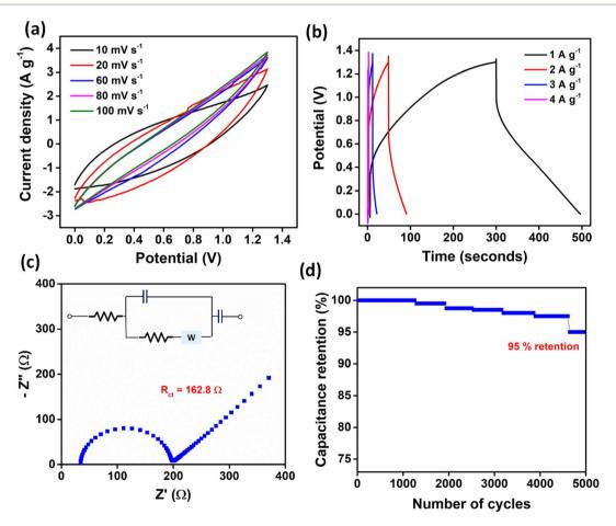
Fig. 6 (a) Cyclic voltammograms of CuNi-PTC at various scan rates, (b) GCD curves at different current densities, (c) Nyquist plot and (d) cycling stability of CuNi-PTC at current density 6 A g $^{-1}$ , using a two-electrode system.
