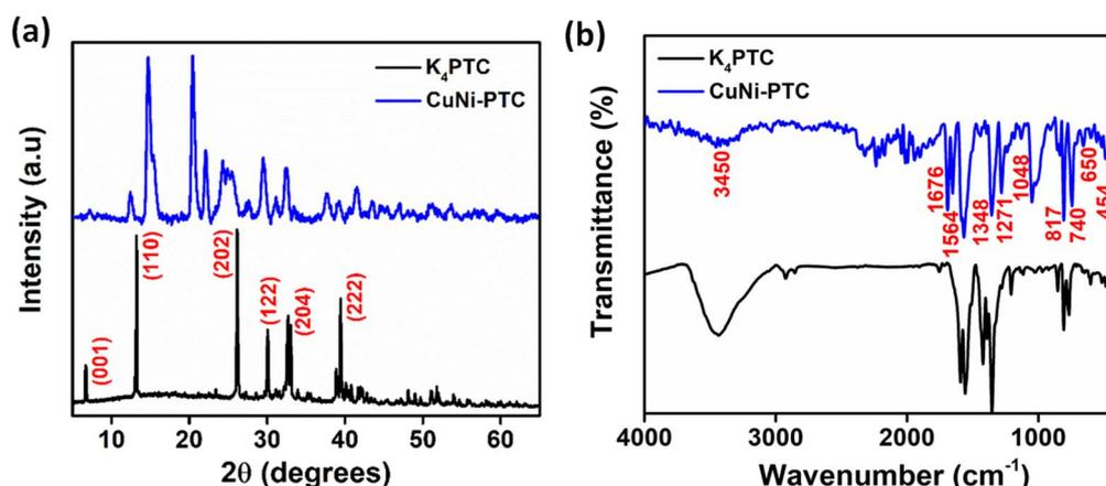
Fig. 1 (a) X-ray diffractogram and (b) FTIR spectra of K<sub>4</sub>PTC and CuNi-PTC.
