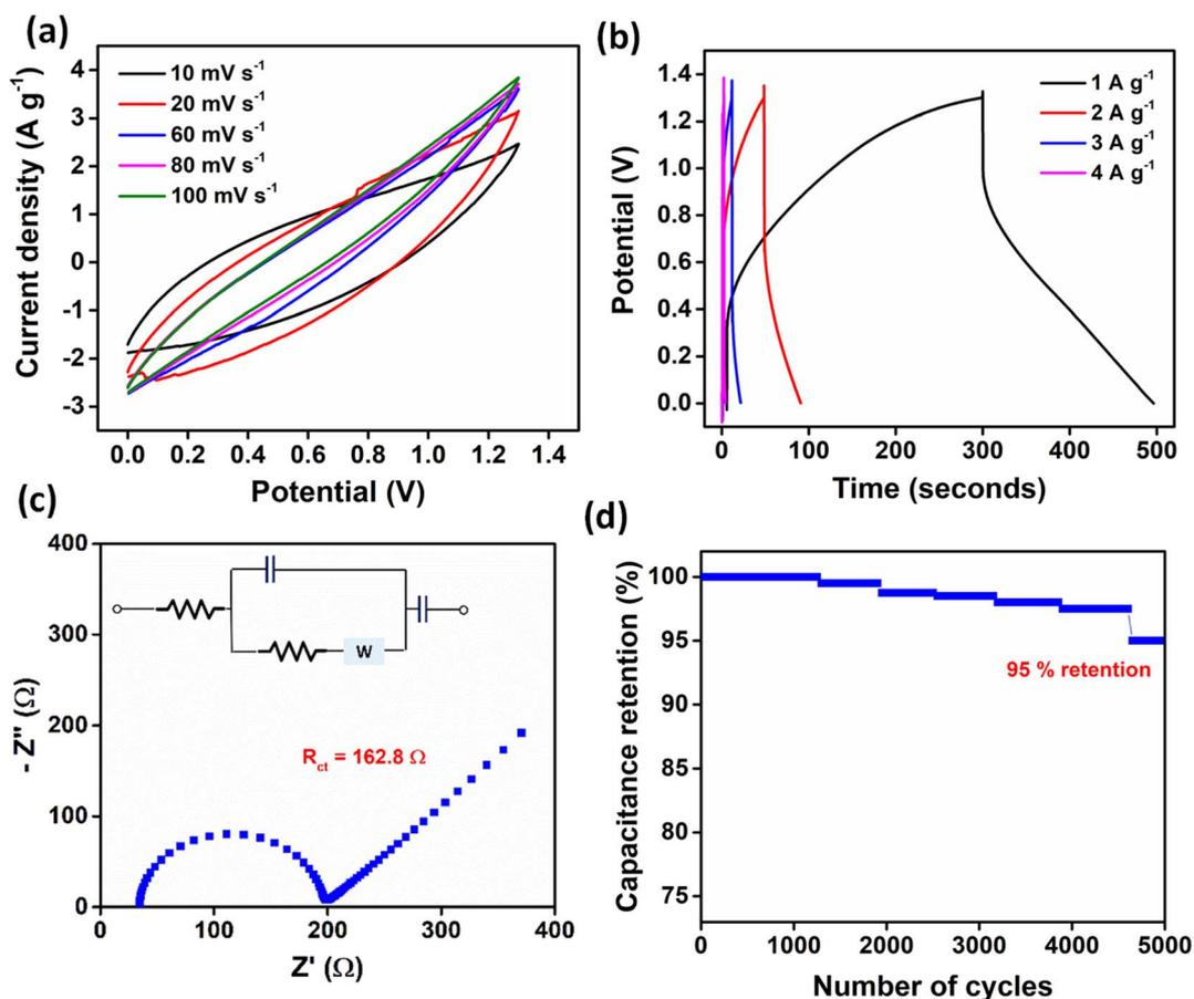
Fig. 6 (a) Cyclic voltammograms of CuNi-PTC at various scan rates, (b) GCD curves at different current densities, (c) Nyquist plot and (d) cycling stability of CuNi-PTC at current density 6  $\text{A g}^{-1}$ , using a two-electrode system.
