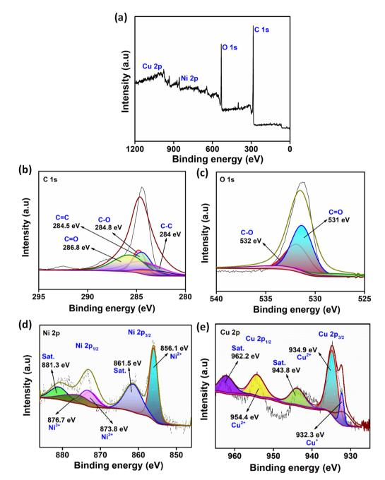
Fig. 2 (a) XPS survey spectrum of CuNi-PTC. High-resolution core spectra of (b) C 1s, (c) O 1s, (d) Ni 2p, and (e) Cu 2p.
