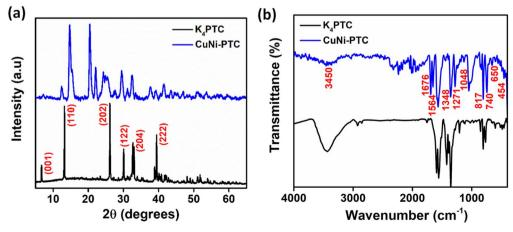
Fig. 1 (a) X-ray diffractogram and (b) FTIR spectra of K₄PTC and CuNi-PTC.
