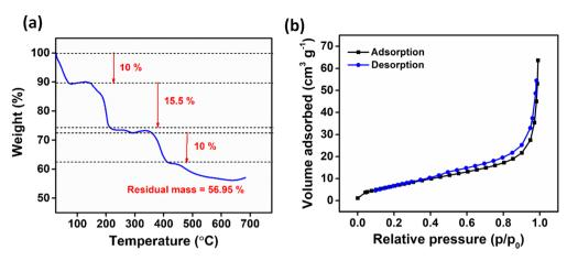
Fig. 4 (a) Thermogram and (b) N<sub>2</sub> adsorption-desorption isotherm of CuNi-PTC
