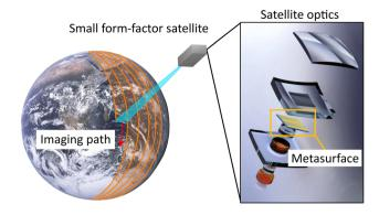
**Fig. 1** Illustration of the proposed satellite system. A small form-factor satellite images a strip of the Earth's surface, forming a complete image over time. A metasurface can be placed within an existing imaging system without increasing the overall footprint. Images reproduced with permission from: NASA, image ID AS17-148-22727; Rob Sharp, CHICO hyperspectral sensor.
