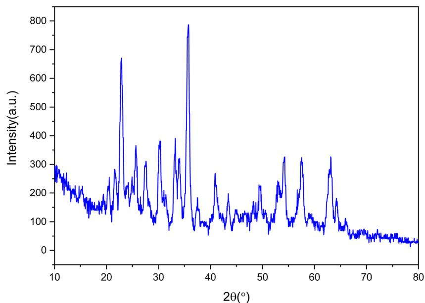
Fig. 2 XRD analysis of Hercynite@SiO<sub>2</sub>-PMA.
