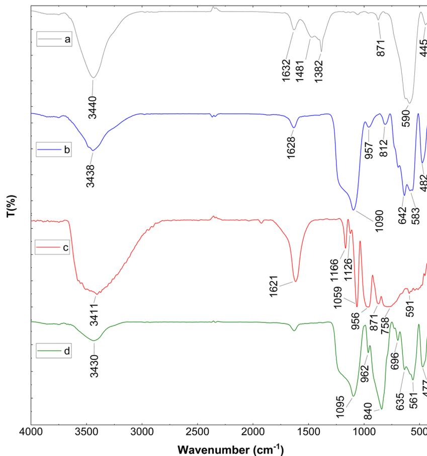
Fig. 1 FT-IR analysis of (a) hercynite, (b) Hercynite@SiO<sub>2</sub>, and (c) pure PMA, (d) Hercynite@SiO<sub>2</sub>-PMA.
