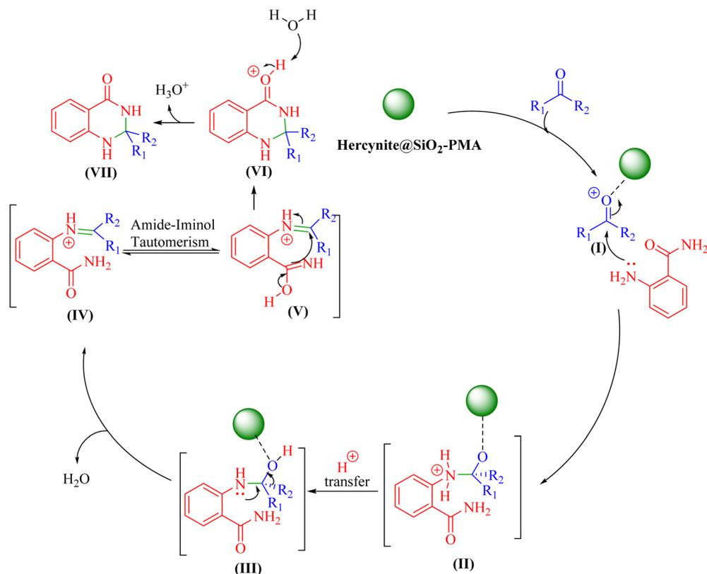
Scheme 2 Possible mechanism for the synthesis of 2,3-dihydroquinazolin-4(1H)-ones over the catalysis of Hercynite@SiO<sub>2</sub>-PMA nanocomposite.
