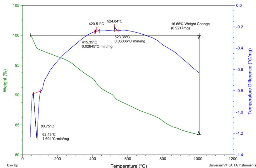
Fig. 3 TGA-DSC curves of Hercynite@SiO<sub>2</sub>-PMA.
