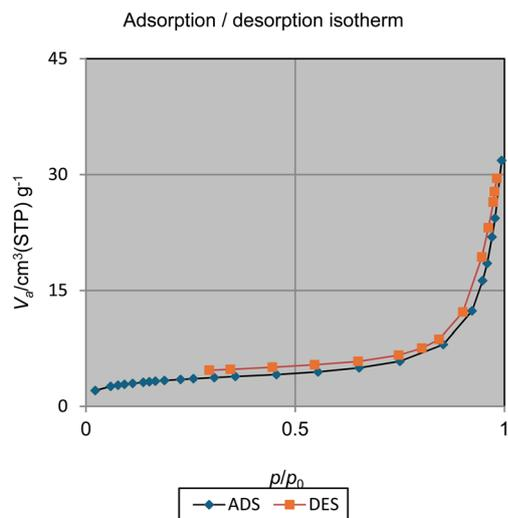
Fig. 9  $N_2$  adsorption/desorption isotherms of Hercynite@SiO<sub>2</sub>-PMA.
