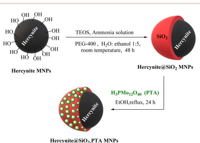
Scheme 1 Stepwise synthesis of Hercynite@SiO<sub>2</sub>-PMA magnetic nanocomposite.
