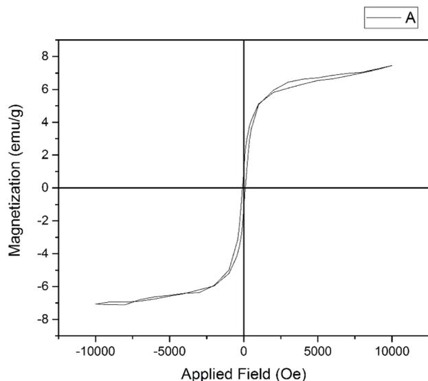
Fig. 8 VSM analysis of Hercynite@SiO<sub>2</sub>-PMA.
