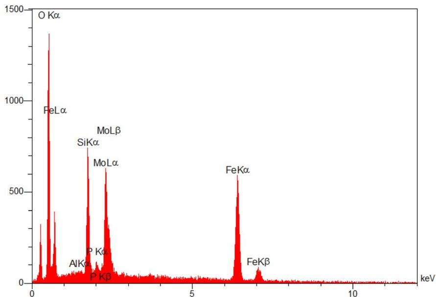
Fig. 4 EDAX analysis of Hercynite@SiO<sub>2</sub>-PMA.
