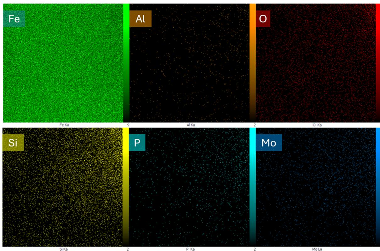
Fig. 5 Elemental mapping images of Hercynite@SiO<sub>2</sub>-PMA.
