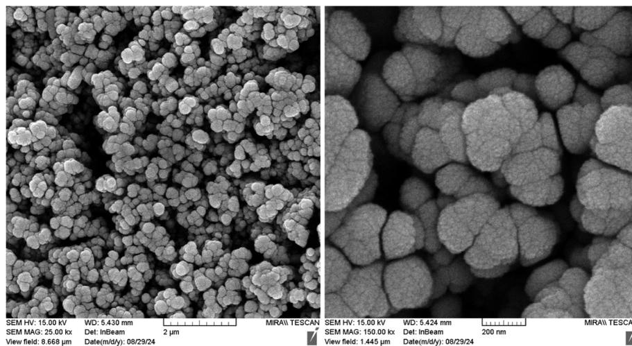
Fig. 6 SEM images of Hercynite@SiO<sub>2</sub>-PMA.
