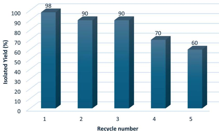
Fig. 10 The reusability of Hercynite@SiO<sub>2</sub>-PMA nanocomposite.
