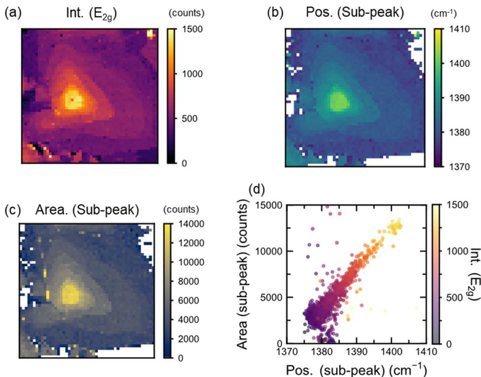
Fig. 2 Raman mappings of hBN  $E_{2g}$  intensity (a), sub-peak position (b) and area of the sub-peak (c). (d) Plot of the area of the sub-peak against its position. The colours of the plots indicate the intensity of the  $E_{2g}$  band. Here, the intensity and area mean the peak height and integrated area of each peak, respectively.
