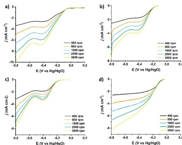
Fig. 7 LSV ORR curves recorded with different rotation speeds (400–3600 rpm) for (a) (7,6)-SWCNTs, and functionalized materials (b) 1, (c) 2, and (d) 3. All assays were performed in  $O_2$ -saturated aqueous 0.1 M KOH as electrolyte with a scan rate of  $5 \text{ mV s}^{-1}$ . The current densities ( $j$ ) are normalized to the electrode surface.
