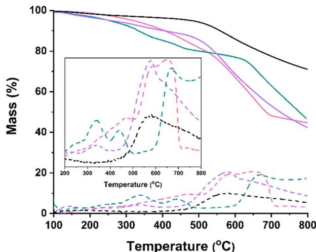
Fig. 4 Thermogravimetric analysis (TGA) graphs recorded under  $N_2$  constant flow of (7,6)-SWCNTs (black), and functionalized materials **1** (purple), **2** (pink), and **3** (green). Dotted lines represent the 1st weight derivatives of each TGA curve. Inset displays a magnified area of the 1st weight derivatives of each material, clearly showcasing the degradation steps.
