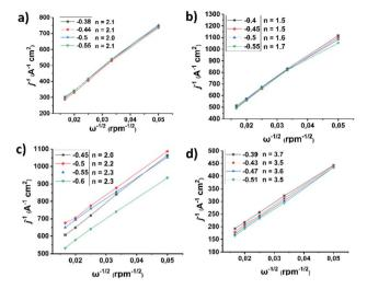
Fig. 8 K–L plots of the ORR LSV curves recorded with different rotation speeds (400-3600 rpm) for (a) (7,6)-SWCNTs, and functionalized materials (b) **1**, (c) **2**, and (d) **3**. All assays were performed in O<sub>2</sub>-saturated aqueous 0.1 M KOH as electrolyte with a scan rate of 5 mV s<sup>-1</sup>. The current densities (j) are normalized to the electrode surface.
