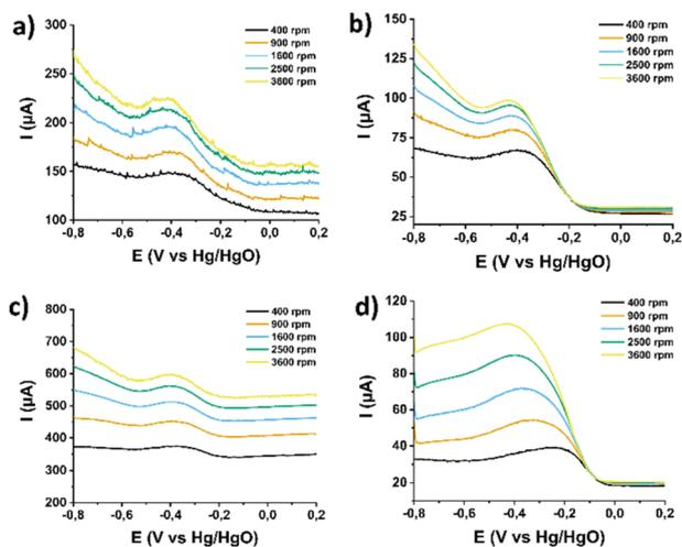
Fig. 9 RRDE response in different rotation speeds (400–3600 rpm) for (a) (7,6)-SWCNTs, and functionalized materials (b) 1, (c) 2, and (d) 3. All assays were performed in  $O_2$ -saturated aqueous 0.1 M KOH as electrolyte with a scan rate of  $5 \text{ mV s}^{-1}$ .
