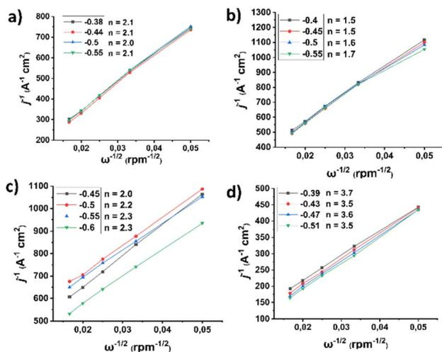
Fig. 8 K–L plots of the ORR LSV curves recorded with different rotation speeds (400–3600 rpm) for (a) (7,6)-SWCNTs, and functionalized materials (b) 1, (c) 2, and (d) 3. All assays were performed in  $O_2$ -saturated aqueous 0.1 M KOH as electrolyte with a scan rate of  $5 \text{ mV s}^{-1}$ . The current densities ( $j$ ) are normalized to the electrode surface.
