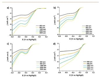
Fig. 7 LSV ORR curves recorded with different rotation speeds (400-3600 rpm) for (a) (7,6)-SWCNTs, and functionalized materials (b) **1**, (c) **2**, and (d) **3**. All assays were performed in  $O_2$ -saturated aqueous 0.1 M KOH as electrolyte with a scan rate of 5 mV s<sup>-1</sup>. The current densities (j) are normalized to the electrode surface.
