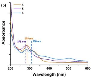
Fig. 1 (a) UV-Vis spectra of (7,6)-SWCNTs (black) and functionalized materials 1 (purple), 2 (pink) and 3 (green). (b) Corresponding UV-Vis spectra of molecular analogues 4 (orange), 5 (deep purple) and 6 (light blue).
