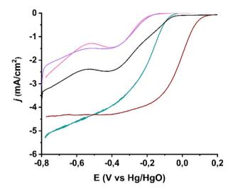
**Fig. 6** LSV ORR curves recorded with a rotation speed of 1600 rpm for (7,6)-SWCNTs (black), and functionalized materials **1** (purple), **2** (pink) and **3** (green), in comparison with the commercially available benchmark catalyst Pd/C (wine). All assays were performed in  $O_2$ -saturated aqueous 0.1 M KOH as electrolyte with a scan rate of 5 mV s $^{-1}$ . The current densities (j) are normalized to the electrode surface.
