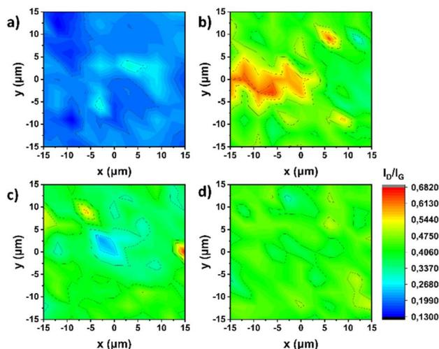
Fig. 3 Raman spectroscopy (514 nm) mappings (scanning area:  $30 \mu\text{m} \times 30 \mu\text{m}$ ) of (a) (7,6)-SWCNTs, and functionalized materials (b) 1, (c) 2, and (d) 3.
