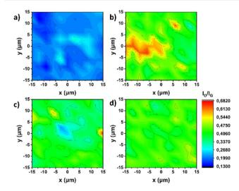
Fig. 3 Raman spectroscopy (514 nm) mappings (scanning area: 30  $\mu$ m imes 30  $\mu$ m) of (a) (7,6)-SWCNTs, and functionalized materials (b) 1, (c) 2, and (d) 3.
