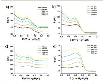
Fig. 9 RRDE response in different rotation speeds (400–3600 rpm) for (a) (7,6)-SWCNTs, and functionalized materials (b) 1, (c) 2, and (d) 3. All assays were performed in  $O_2$ -saturated aqueous 0.1 M KOH as electrolyte with a scan rate of 5 mV s<sup>-1</sup>.
