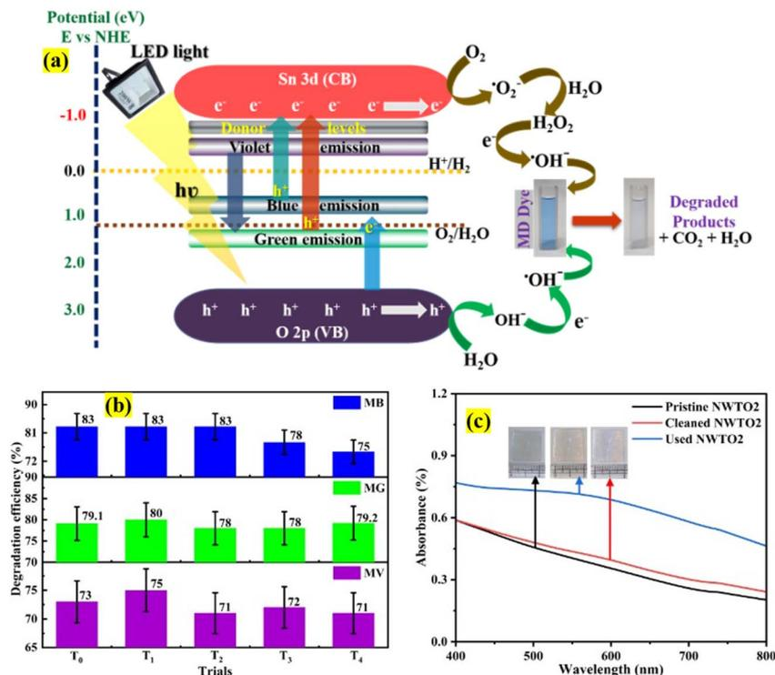
Fig. 10 (a) Plausible charge transfer mechanism for the MD dye degradation, (b) recyclability test showing variation in disintegration efficiency from the pristine (T<sub>0</sub>) attempt to four re-use trials (T<sub>1</sub> to T<sub>4</sub>) and (c) absorbance spectrum of the as-prepared, used, and cleaned surface following the photocatalytic reaction with the NWTO2 catalyst. The standard error is also denoted.
