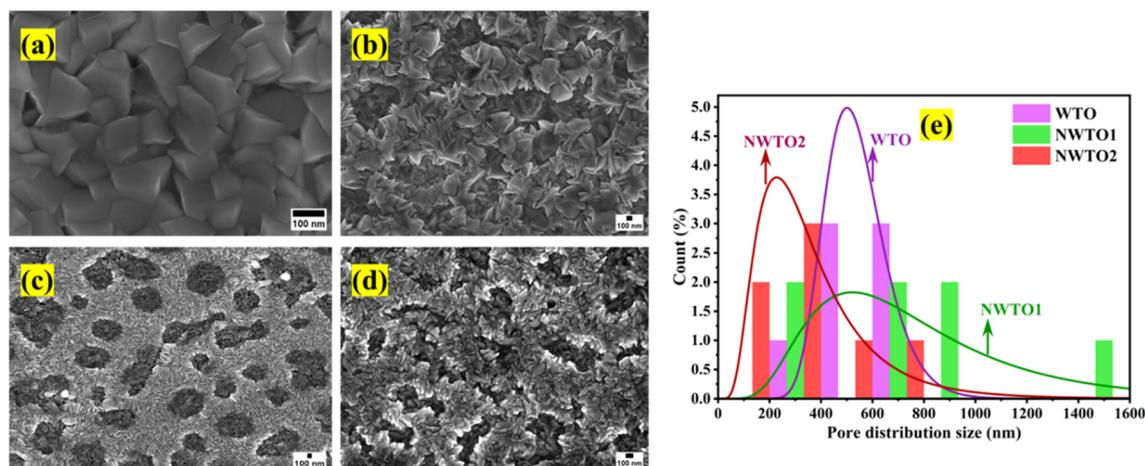
Fig. 2 Field emission scanning electron micrographs of the spray-pyrolyzed pure and Nb:W co-doped SnO<sub>2</sub> films (a–d) indicating variation in the surface features and pore size distribution plot for the doped films (e).
