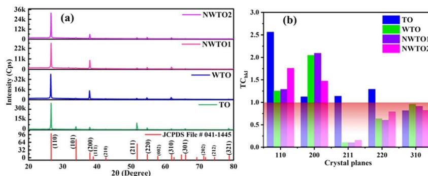
Fig. 1 (a) XRD plots compared with the standard JCPDS file, and (b) texture co-efficient values of spray pyrolyzed Nb and W co-doped SnO<sub>2</sub> films.
