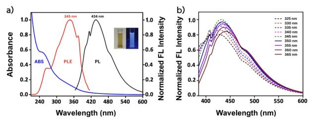
Fig. 1 (a) UV-vis absorption (blue curve), PL excitation (red curve), and PL emission spectra (black curve) of HC-CQDs (inset: pictures of HC-CQDs in ambient (left) and UV light (right)). (b) Emission spectra of HC-CQDs recorded under excitation wavelengths ranging from 325 to 365 nm.
