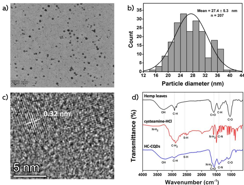
Fig. 2 (a) TEM image of HC-CQDs; (b) particle size distribution of HC-CQDs; (c) HR-TEM image of HC-CQDs; and (d) FT-IR spectra of raw hemp, cysteamine-HCl, and synthesized HC-CQDs.
