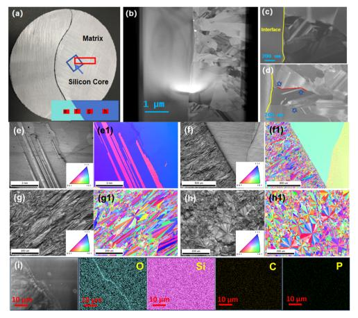
Fig. 2 (a-d) The twin structures within the polycrystalline silicon matrix, as observed under an aberration-corrected electron microscope; (e-e1)SEM-EBSD images of the polysilicon core; (f-f1) SEM-EBSD of the polysilicon interface; (g-h1) SEM-EBSD EBSD of the polysilicon matrix; (i) SEM-EDS image of the polysilicon interface.
