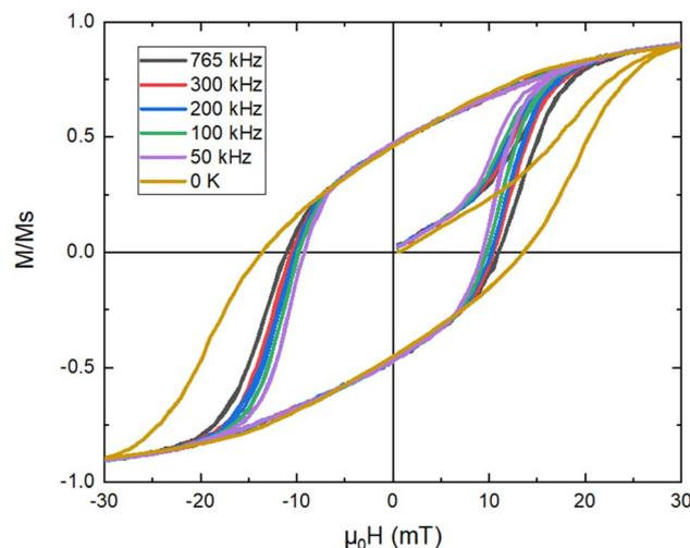
Fig. 8 AC hysteresis loops for 30 mT magnetic field amplitude and for various frequencies (50–765 kHz). The largest loop corresponds to 0 K and is independent of the frequency.<sup>35</sup>
