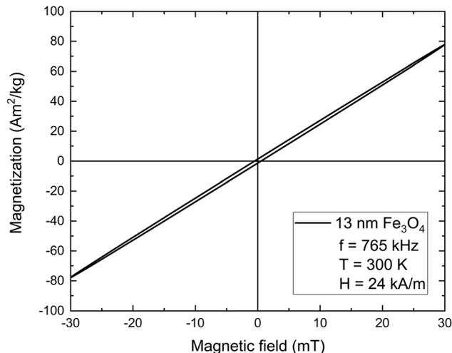
Fig. 14 Hysteresis loop for non-interacting magnetite nanoparticles of diameter 13 nm. The applied magnetic field amplitude and the bulk saturation magnetization are equal to  $24 \text{ kA m}^{-1}$  (30 mT) and  $91 \text{ A m}^2 \text{ kg}^{-1}$  ( $480 \text{ kA m}^{-1}$ ). From the shape of the loop, it is revealed that the linear relationship between magnetization and the applied magnetic field is reasonable approximation.
