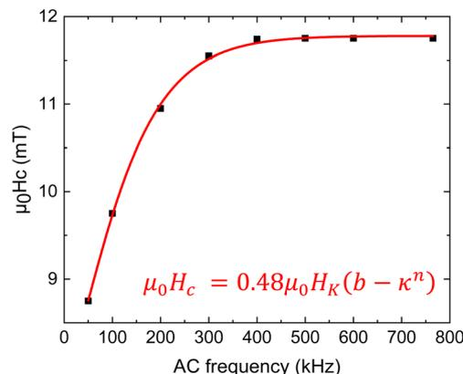
Fig. 9 Dependence of the hysteresis loop with frequency and fitting of obtained data. The fitting curve and the corresponding equation are shown with red color.<sup>35</sup>
