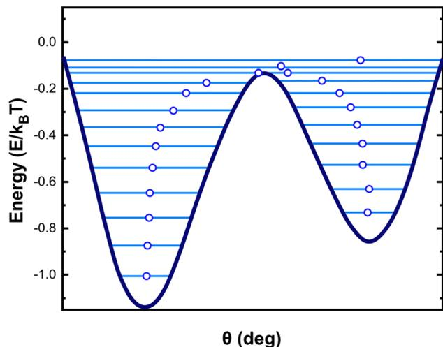
Fig. 7 Schematic diagram of additional energy states emerged for a DW magnetic nanoparticle when thermal field is activated in the micromagnetic approach.<sup>45</sup>
