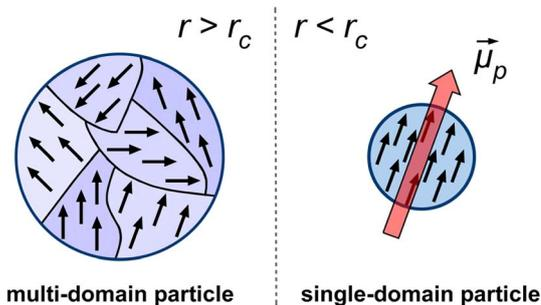
Fig. 1 Schematic representation of magnetic domain structures in nanoparticles based on their size. Particles with a radius  $r$  larger than a critical value  $r_c$  exhibit a multi-domain structure (left), where multiple magnetic domains are separated by domain walls. When the particle radius is smaller than  $r_c$ , it becomes a single-domain particle (right), where all atomic spins align coherently, resulting in a net magnetic moment  $\vec{\mu}_p$  in a single direction.<sup>43</sup>
