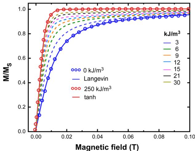
Fig. 5 Monte Carlo simulation resulted curves of magnetization of  $\text{Fe}_3\text{O}_4$  magnetic nanoparticle with diameter 40 nm versus external field varied from 0 to 0.1 T and for different values of the effective anisotropy. The magnetic field is applied along the easy axis ( $\varphi = 0$ ).<sup>45</sup>
