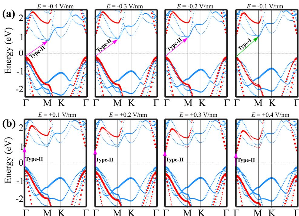
Fig. 9 (a) Weighted projections of the band structures of the GeH/SiSb heterostructure under (a) negative and (b) positive electric fields. The weighted projections of the GeH and SiSb layers are denoted by red and blue circles, respectively. Green and purple arrows represent the type-I and type-II band alignments of the heterostructure.
