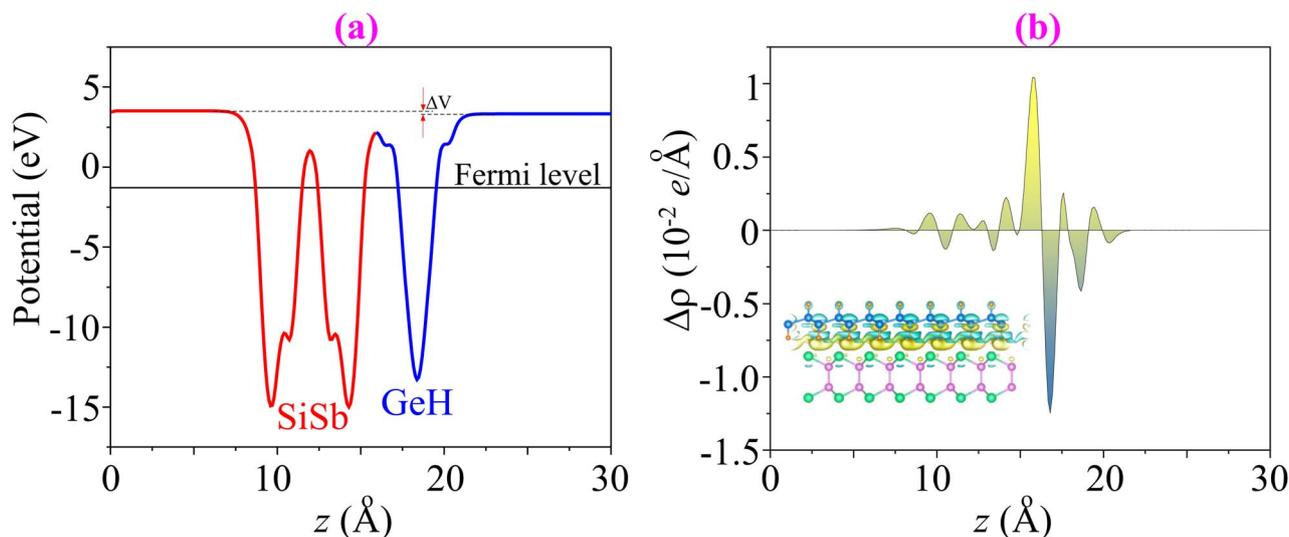
Fig. 7 (a) Electrostatic potential and (b) charge density difference of the GeH/SiSb heterostructure. The 3D isosurface of the GeH/SiSb heterostructure is displayed in the inset, where the accumulation and depletion of charges are visualized by yellow and cyan colors.
