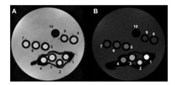
Fig. 4 Representative  $T_{\rm 2w}$  (A) and  $T_{\rm 1w}$  (B) MR images of phantoms composed by glass capillaries filled with the Fe-NPs at variable iron concentration, as follows: (1) 1 mM, (2) 0.7 mM, (3) 0.5 mM, (4) 0.3 mM, (5) 0.2 mM, (6) 0.1 mM, (7) 0.05 mM, (8) 0.03 mM, (9) 0.02 mM and (10) empty reference capillary ( $B_0 = 7.1$  T).
