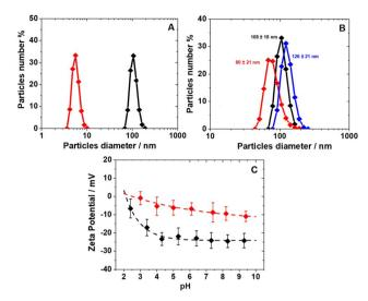
Fig. 2 (A) DLS profiles of PEG (black,  $[Fe^{3+}] = 0.17 \text{ mM}$ ) and PVP/Fe(III) – GA NPs (red,  $[Fe^{3+}] = 0.06$  mM) in water at pH 7.4; (B) DLS of PEG/ Fe(III)-GA NPs at pH 3.4 (red), 7.4 (black) and 8.8 (blue); (C) ζ-potential data for PEG (black) and PVP/Fe(III)-GA (red) as a function of pH.
