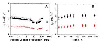
Fig. 5 (A)  $^{1}$ H NMRD profiles at 298 K of PEG/Fe(III)-GA ([Fe $^{3+}$ ] = 1.7 mM) (black) and PVP/Fe(III)-GA ([Fe<sup>3+</sup>] = 0.6 mM) (red) in water (full symbols) and in Seronorm™ solution (empty symbols). (B) Dependence of  ${}^{1}H$   $r_{1}$  over time for PEG/Fe(III) – GA (black) and PVP/Fe(III) – GA (red) in Seronorm™ at 310 K.
