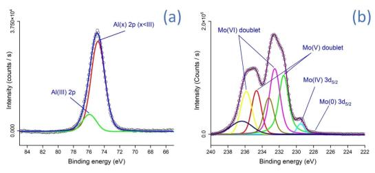
Fig. 5 X-ray photoelectron spectroscopy of (a)  $AlO_x$  and (b)  $MoO_x$
