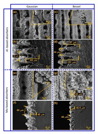
Fig. 3 (a-d) SEM micrographs of Al samples structured with femtosecond Gaussian and Bessel beams: (a and c) top views with zoomedin insets, and (b and d) the corresponding cross-sectional views. (e-h) SEM micrographs of Mo structured with femtosecond Gaussian and Bessel beams: (e and g) top views with zoomed-in insets, and (f and h) the corresponding cross-sectional views.
