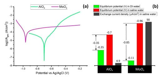
Fig. 10 Comparison of the (a) Tafel plots in saline water and (b) the corresponding rest potentials (in saline as well as DI water) and exchange current densities of structured AlO<sub>x</sub> and MoO<sub>x</sub> samples.
