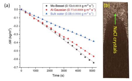
Fig. 8 (a) Water evaporation in the dark normalized to geometric surface area vs. time. Linear fitting was applied to extract the slope which is the geometric area normalized evaporation rate ( $\dot{m}_{\rm geo}$ ). (b) A camera captured image of MoO<sub>x</sub> (i.e., Mo-Bessel) after 1.4 hours of evaporation in the dark.
