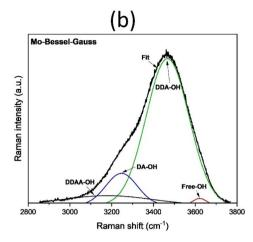
Fig. 9 Deconvoluted OH stretching vibration in the Raman spectra for (a) Al-Gaussian and (b) Mo-Bessel-Gauss (with DAA-OH percentage zero) in 3.5 wt% NaCl solution.
