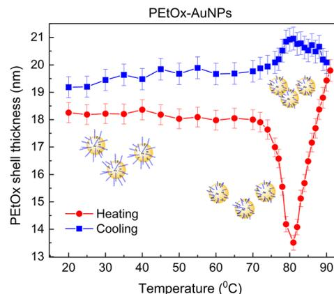
Fig. 2 Temperature dependence of DLS derived PEtOx shell thickness of PEtOx-AuNPs during the heating-cooling cycle in the temperature range 20–91–20 °C.
