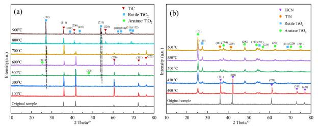
Fig. 4 X-ray diffraction pattern of samples after oxidation at different temperatures: TiC (a) and TiCN (b).
