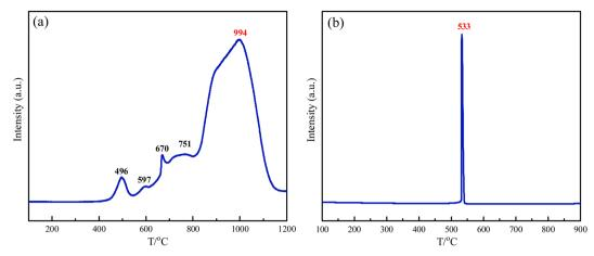
Fig. 5 TPO-IR curves of undoped samples TiC (a) and TiCN (b).
