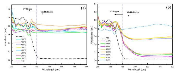
Fig. 9 UV-Vis DRS spectra of TiC (a) and TiCN (b).
