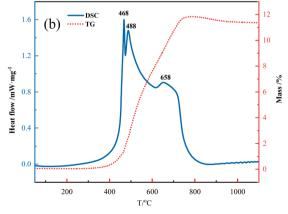
Fig. 6 TG and DSC curves of TiC (a) and TiCN (b).
