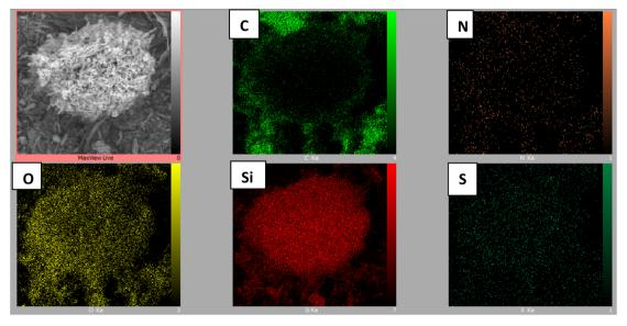
Elemental mapping of the PABSA-Pr-PMO nanocatalyst (1)
