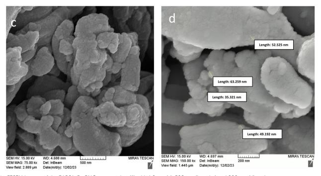
Fig. 3 FESEM images of the PABSA-Pr-PMO nanocatalyst (1) with 1.0 μm (a), 500 nm (b and c) and 200 nm (d) scales.
