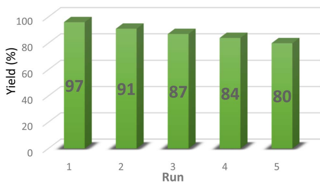
Fig. 9 Reusability data for the PABSA-Pr-PMO nanocatalyst (1) in the synthesis of 5a.
