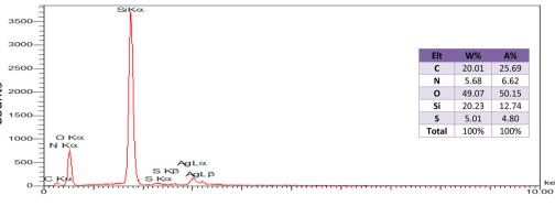
Fig. 5 The EDX spectrum of the PABSA-Pr-PMO nanocatalyst (1).
