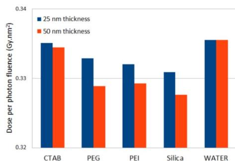
Fig. 2 Dose normalized to incident photon fluence for different coating materials with 25 nm and 50 nm thicknesses.
