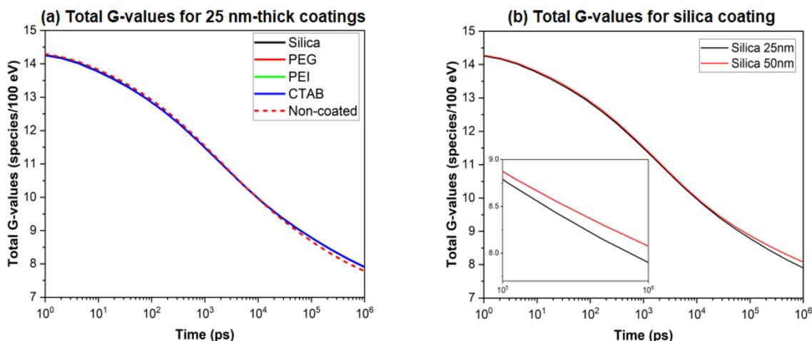
Fig. 5 Total G-values for different coatings with 50 nm thickness (a), and silica coating with two thicknesses (b). The inset in (b) provides a magnified view of the time interval from 100 ns to 1  $\mu$ s.
