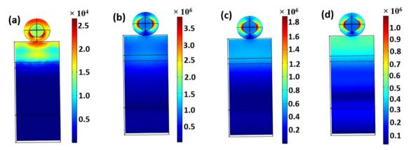
Fig. 3 Electric field profiles for TiN/SiO<sub>2</sub> core/shell decorated PSC with a core radius of 50 nm at different wavelengths: (a) 300 nm, (b) 800 nm, (c) 1000 nm, and (d) 1200 nm.
