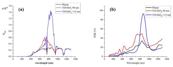
Fig. 5 (a) Optical carrier generation rate ( $G_{opt}$ ) and (b) normalized light absorption profiles for planar and TiN/SiO<sub>2</sub>-decorated PSCs.
