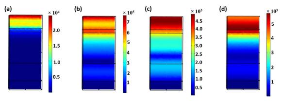
Fig. 2 Electric field profiles at different wavelengths: (a) 300 nm, (b) 800 nm, (c) 1000 nm, and (d) 1200 nm for planar PSCs.
