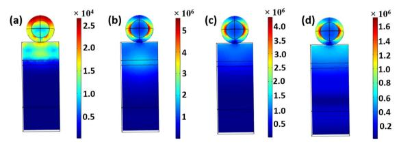
Fig. 4 Electric field profiles for  $TiN/SiO_2$  core/shell decorated PSC with a core radius of 75 nm at different wavelengths: (a) 300 nm, (b) 800 nm, (c) 1000 nm, and (d) 1200 nm.
