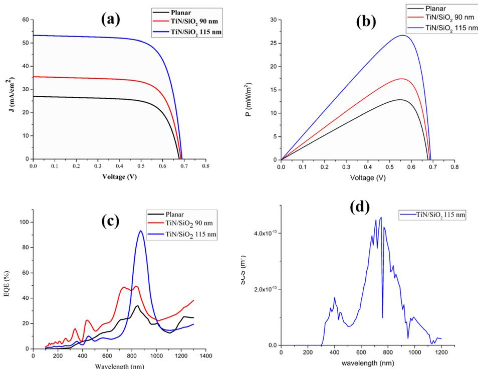
Fig. 6 (a)  $J$ - $V$ , (b)  $P$ - $V$ , (c) EQE, and (d) SCS characteristics of proposed TiN/SiO<sub>2</sub>-decorated PSCs.
