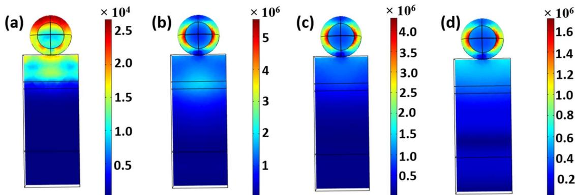
Fig. 4 Electric field profiles for TiN/SiO<sub>2</sub> core/shell decorated PSC with a core radius of 75 nm at different wavelengths: (a) 300 nm, (b) 800 nm, (c) 1000 nm, and (d) 1200 nm.
