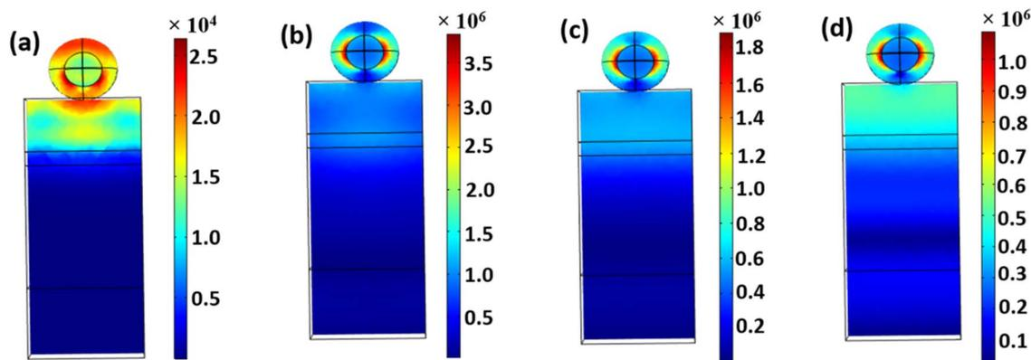
Fig. 3 Electric field profiles for TiN/SiO<sub>2</sub> core/shell decorated PSC with a core radius of 50 nm at different wavelengths: (a) 300 nm, (b) 800 nm, (c) 1000 nm, and (d) 1200 nm.
