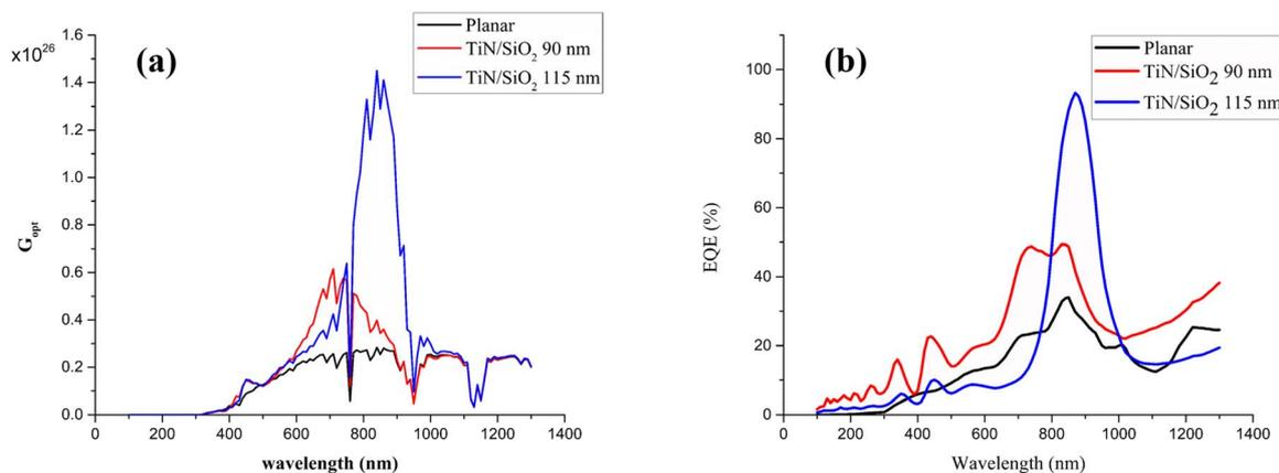
Fig. 5 (a) Optical carrier generation rate ( $G_{opt}$ ) and (b) normalized light absorption profiles for planar and TiN/SiO<sub>2</sub>-decorated PSCs.
