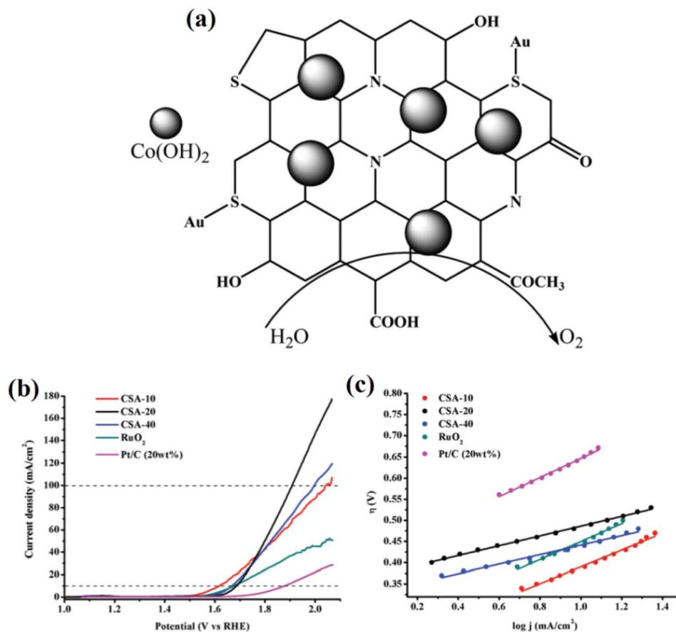
Fig. 3 (a) Schematic diagram of OER activity enhancement by  $\text{Co}(\text{OH})_2$  incorporated Au-doped carbon quantum dots (Au-SCQDs), (b) LSV curve for OER studies, and (c) Tafel plots of  $\text{Co}(\text{OH})_2$ -Au-SCQDs. Reproduced from ref. 51 with permission from the Royal Society of Chemistry.
