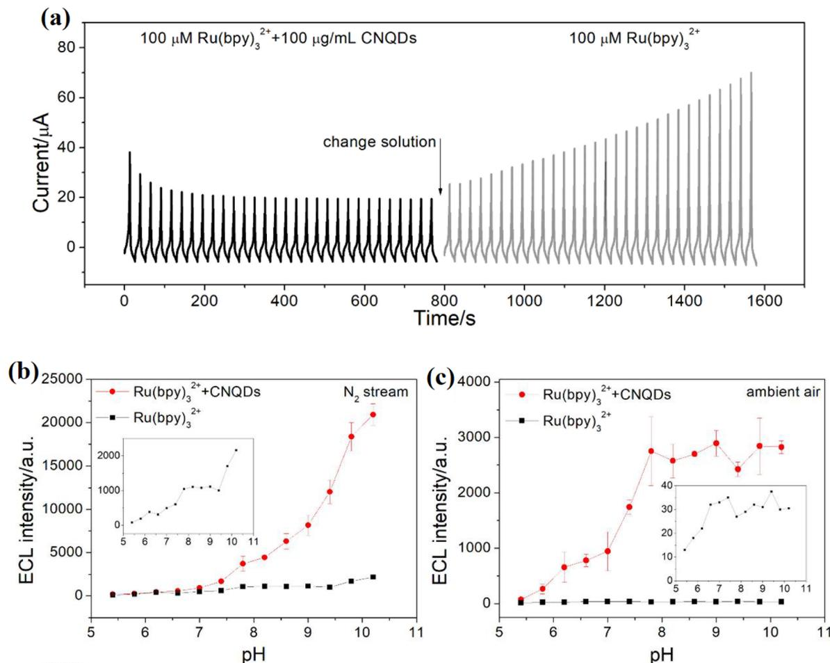
Fig. 4 (a) Chronoamperometric ECL response of Ru(bpy)<sub>3</sub><sup>2+</sup> with and without CNQDs during solution exchange. pH-dependent ECL intensity of Ru(bpy)<sub>3</sub><sup>2+</sup> with and without CNQDs under N<sub>2</sub> (b) and ambient air (c) atmospheres, highlighting enhanced emission with CNQDs, especially at alkaline pH. Reproduced with permission from ref. 59, copyright 2020 American Chemical Society.
