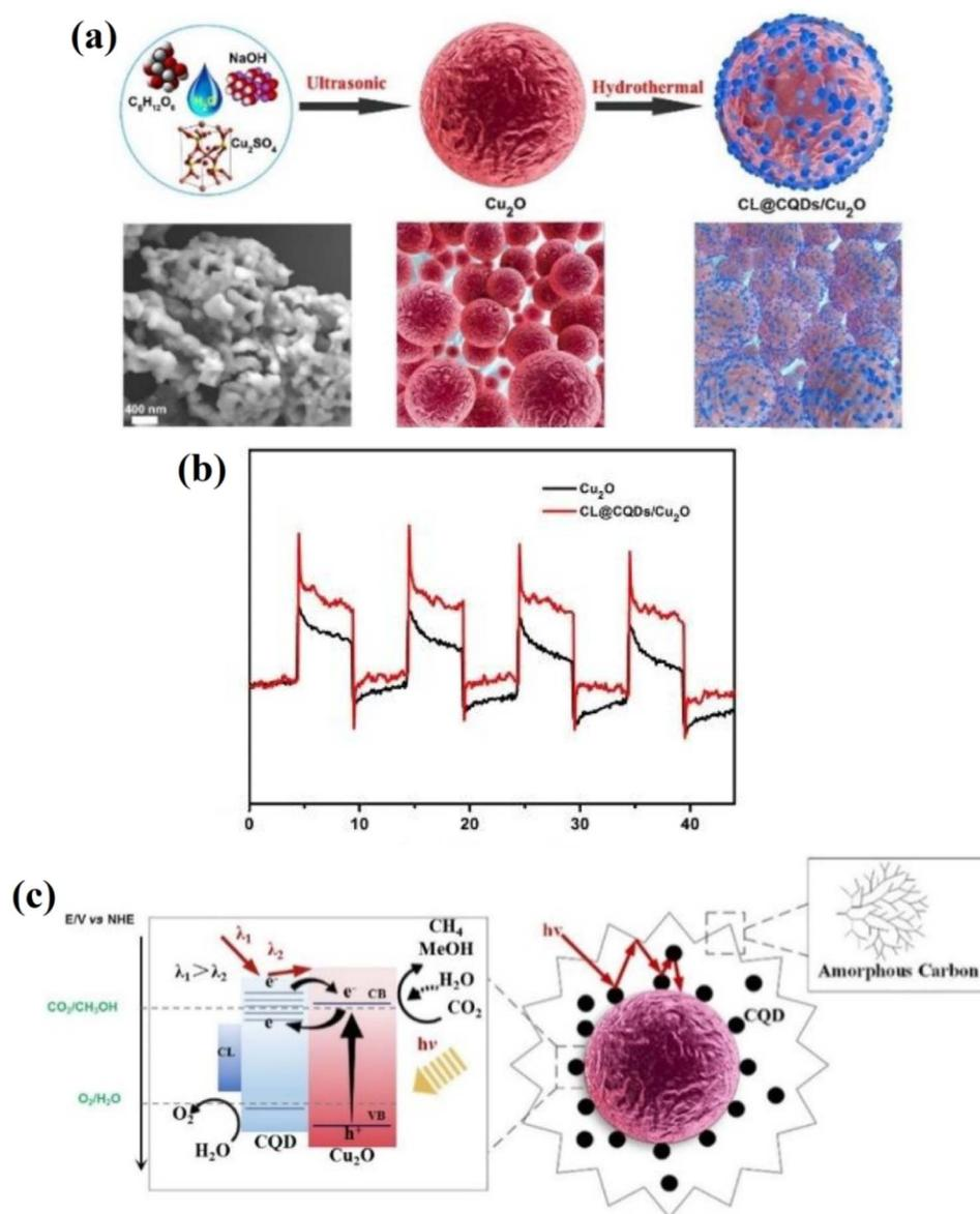
Fig. 7 (a) Synthesis scheme of  $CL@CQDs/Cu_2O$  (bottom left: SEM image). (b) Photocurrent properties of  $Cu_2O$  and  $CL@CQDs/Cu_2O$  in Ar saturated solutions. (c) Proposed photocatalytic  $CO_2$  reduction mechanism on  $CL@CQDs/Cu_2O$ . Reproduced from ref. 109 with permission from the Royal Society of Chemistry.
