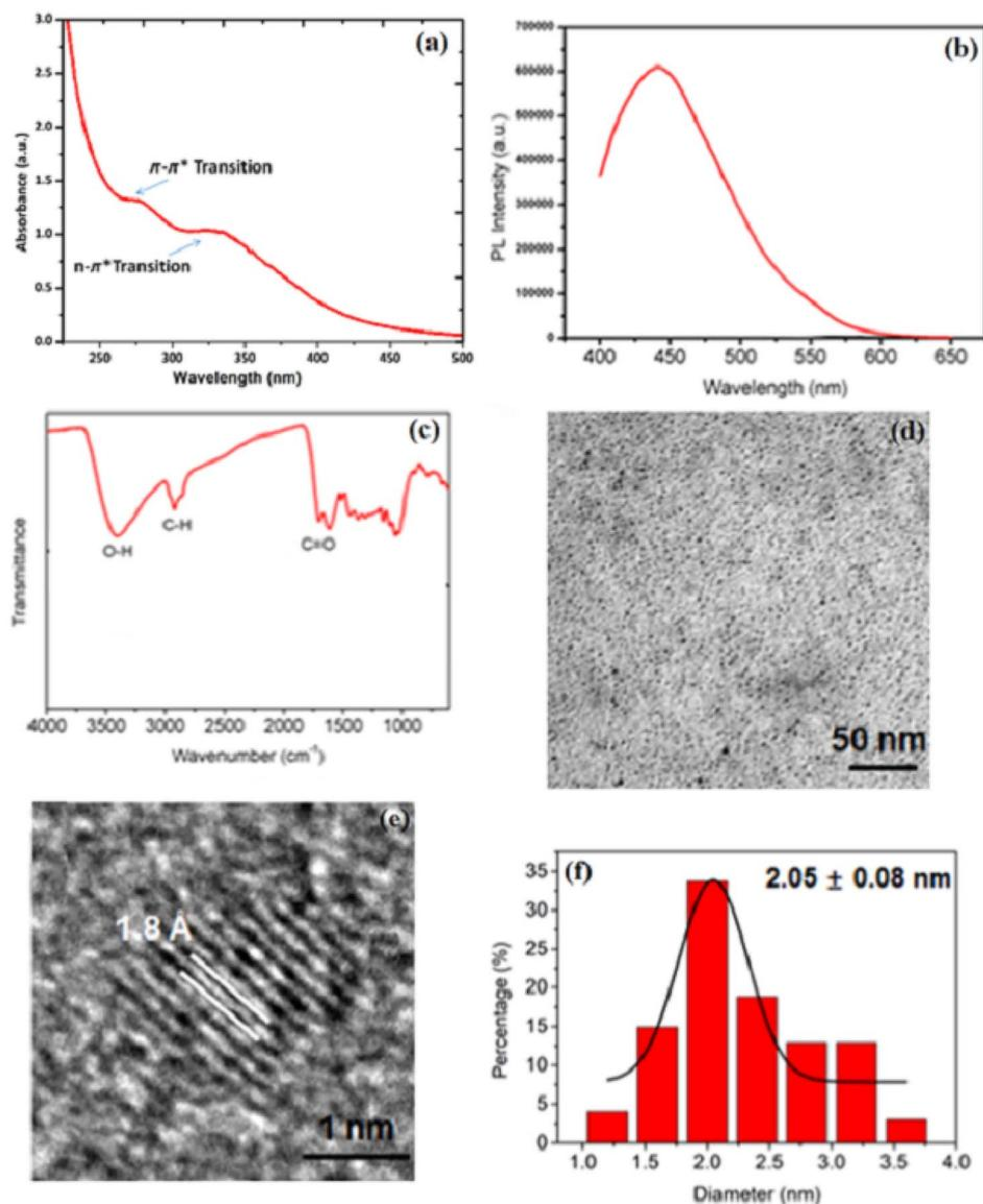
Fig. 1 (a) Structural characterization of CQDs. (b) The photoluminescence (PL) spectra of CQDs at  $10 \mu\text{g mL}^{-1}$  under natural light irradiation. (c) The FTIR spectra of CQDs. Morphological characterization of CQDs. Low and high-resolution TEM images and particle size distributions of (d–f) CQDs. Reproduced from Fu *et al.* (2023),<sup>16</sup> *Heliyon*, under the terms of the Creative Commons Attribution License (CC BY 4.0).
