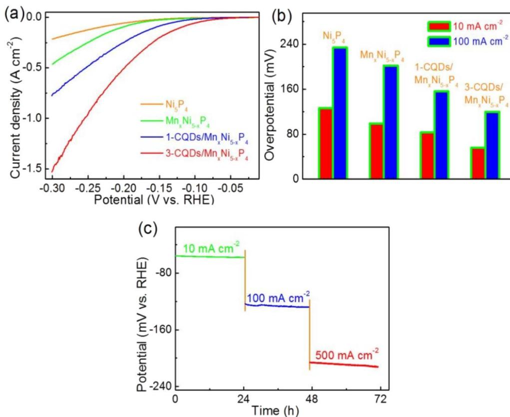
Fig. 6 Electrocatalytic performance of different catalysts in 1 M KOH. (a) Polarization curves, (b) overpotentials at current densities of 10 and 100 mA cm<sup>-2</sup>, and (c) chronopotentiometry curves of 3-CQDs/Mn<sub>x</sub>Ni<sub>5-x</sub>P<sub>4</sub> at different current densities for the HER. Reproduced from ref. 66 with permission from the Royal Society of Chemistry.
