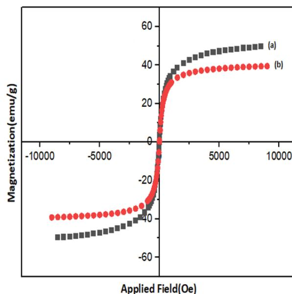
Fig. 6 VSM analysis of (a) Fe<sub>3</sub>O<sub>4</sub> NPs, and (b) nano guar gum/BF<sub>3</sub>/Fe<sub>3</sub>O<sub>4</sub>.
