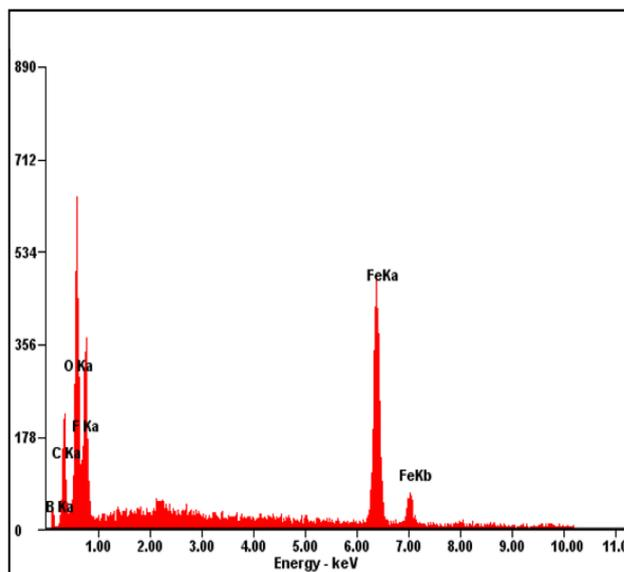
Fig. 7 EDS diagram of nano guar gum/BF<sub>3</sub>/Fe<sub>3</sub>O<sub>4</sub>.
