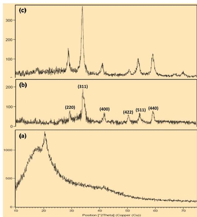
Fig. 5 XRD patterns of (a) guar gum (b) Fe<sub>3</sub>O<sub>4</sub> NPs, and (c) Fe<sub>3</sub>O<sub>4</sub>/guar gum/BF<sub>3</sub>.
