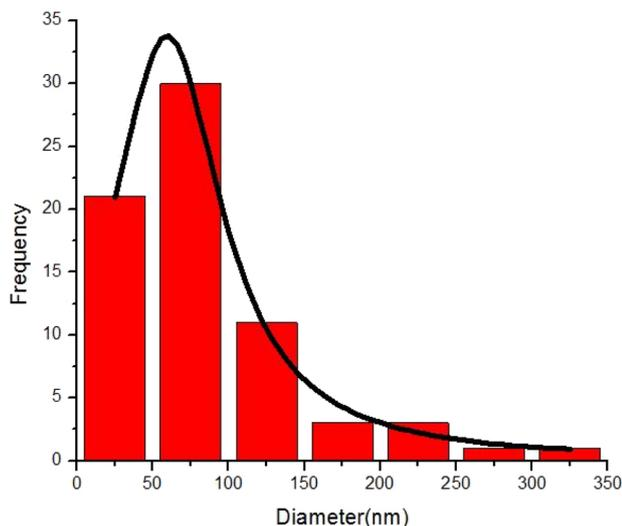
Fig. 3 Particle size distribution histogram nano guar gum/BF<sub>3</sub>/Fe<sub>3</sub>O<sub>4</sub>.
