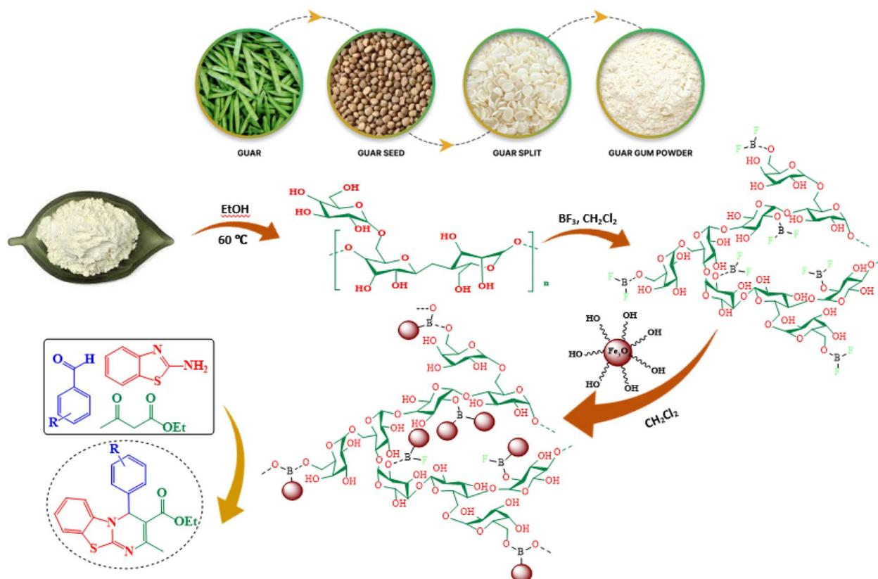
Scheme 1 Preparation of nano guar gum/BF<sub>3</sub>/Fe<sub>3</sub>O<sub>4</sub> for the synthesis of 4*H*-pyrimido[2,1-*b*]benzothiazoles.
