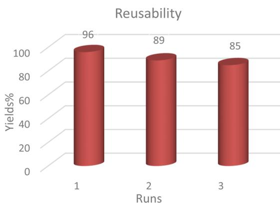
Fig. 10 Reusability of nano guar gum/BF<sub>3</sub>/Fe<sub>3</sub>O<sub>4</sub> for the synthesis of 4*H*-pyrimido[2,1-*b*]benzothiazoles.
