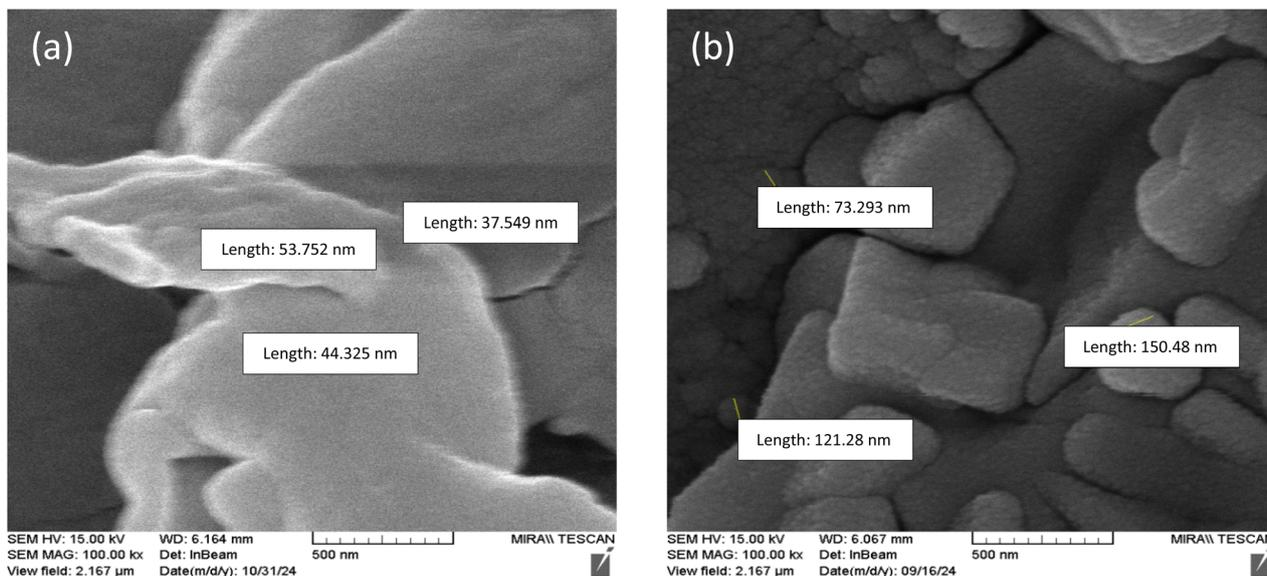
Fig. 2 FESEM images of (a) guar gum, and (b) nano guar gum/BF<sub>3</sub>/Fe<sub>3</sub>O<sub>4</sub>.
