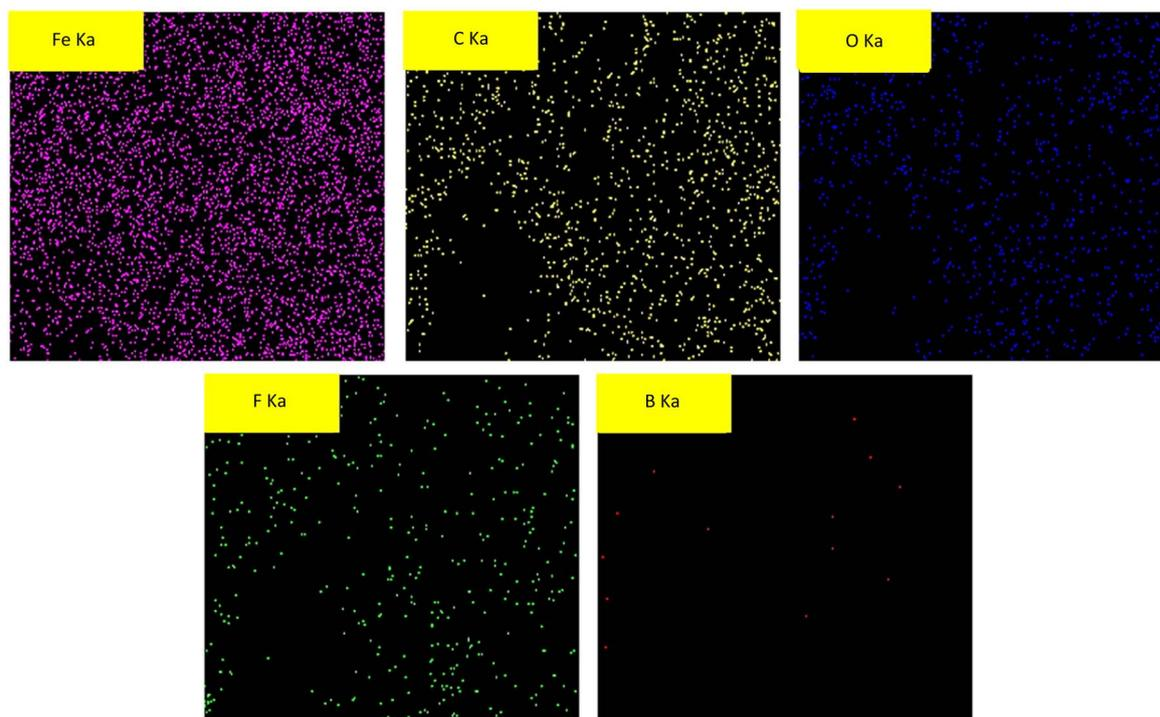
Fig. 8 Maps of nano guar gum/BF<sub>3</sub>/Fe<sub>3</sub>O<sub>4</sub>.
