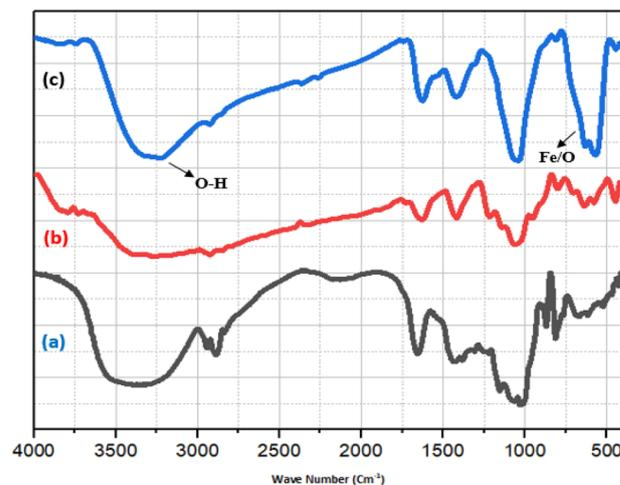
Fig. 1 FT-IR spectra of (a) guar gum, (b) nano guar gum/BF<sub>3</sub>, and (c) nano guar gum/BF<sub>3</sub>/Fe<sub>3</sub>O<sub>4</sub>.
