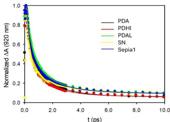
Fig. 6 Ultrafast transient absorption traces upon excitation at 665 nm of PDA NPs, PDAL NPs, DHI NPs, Sepia NPs and SN. Fittings of the experimental data according to a tri-exponential decay model are plotted as continuous lines. Parameters resulting from the fitting are also shown in the table together with the fluorescence quantum yields.
