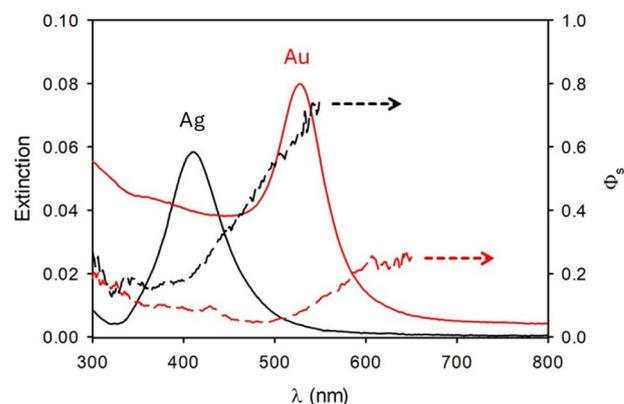
Fig. 3 Extinction (continuous lines) and scattering (dashed lines) spectra of Ag NPs and Au NPs. The results show that extinction in the maximum of the plasmonic band (410 nm for silver and 528 nm for gold) is mostly due to light absorption.
