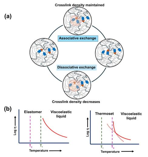
Fig. 1 (a) Associative and dissociative bond exchange reaction in a vitrimer matrix, (b) idealised viscosity vs. temperature curve for vitrimer matrix when  $T_q < T_v$  and  $T_q > T_v$ .
