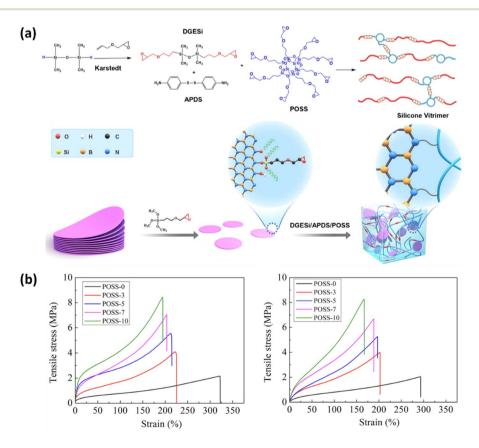
Fig. 6 (a)Schematic diagram for the preparation of the silicone vitrimer matrix and nanocomposite, (b) stress-strain curve for before and after healing of the silicone vitrimer reinforced with different POSS contents. Reproduced with permission from ref. 211 Copyright 2022 Elsevier Inc.
