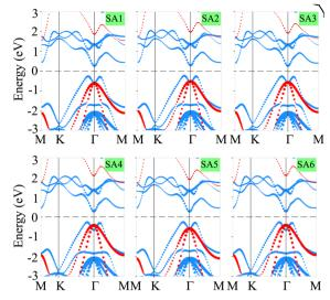
Fig. 3 The weighted projections of the band structures for the SiH/ $\gamma$ -GeSe heterostructure in six different configurations. The SiH and  $\gamma$ -GeSe layers are represented by red and blue lines, respectively, to indicate their contributions
