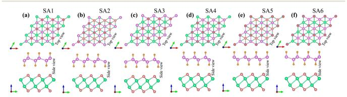
Fig. 1 Different stacking arrangements of the SiH/γ-GeSe heterostructure of (a) SA1, (b) SA2, (c) SA3, (d) SA4, (e) SA5 and (f) SA6
