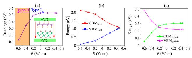
The variations in (a) band gap of the SiH/ $\gamma$ -GeSe heterostructure and (b) the band edges of SiH and (c) band edges of  $\gamma$ -GeSe layers.
