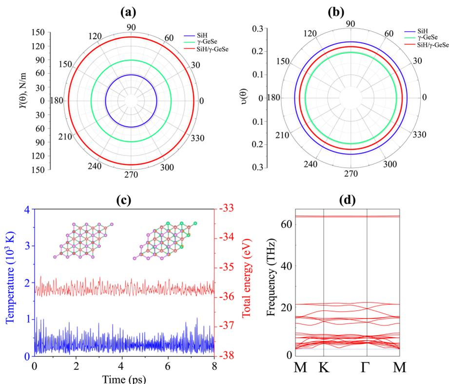
Fig. 4 Angular dependence of the (a) Young modulus and (b) Poisson ration of the SiH/ $\gamma$ -GeSe heterostructure. (c) The variations in the total energy and temperature and (d) the phonon spectra of the SiH/ $\gamma$ -GeSe heterostructure for the most favorable SA2 arrangement.
