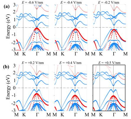
The weighted projections of the band structures of the SiH/ $\gamma$ -GeSe heterostructure under (a) negative-E and (b) positive-E.
