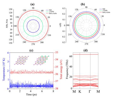
Fig. 4 Angular dependence of the (a) Young modulus and (b) Poison ration of the SiH/ $\gamma$ -GeSe heterostructure. (c) The variations in the total energy and temperature and (d) the phonon spectra of the SiH/ $\gamma$ -GeSe heterostructure for the most favorable SA2 arrangement.
