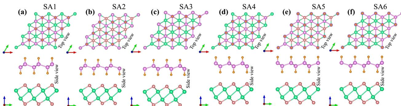
Fig. 1 Different stacking arrangements of the SiH/ $\gamma$ -GeSe heterostructure of (a) SA1, (b) SA2, (c) SA3, (d) SA4, (e) SA5 and (f) SA6.
