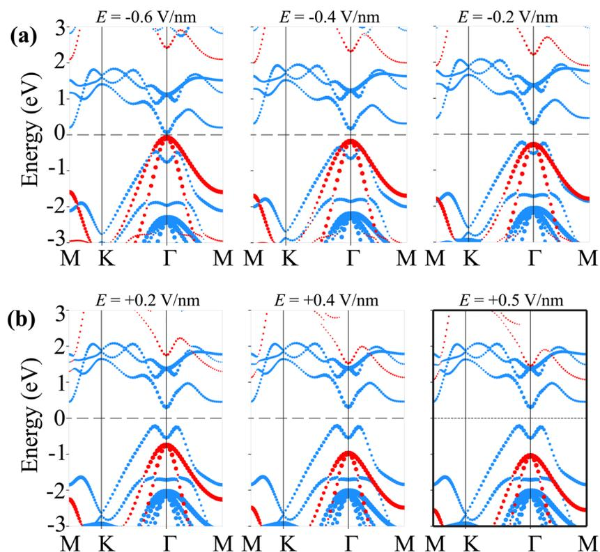
Fig. 8 The weighted projections of the band structures of the SiH/ $\gamma$ -GeSe heterostructure under (a) negative- $E$  and (b) positive- $E$ .
