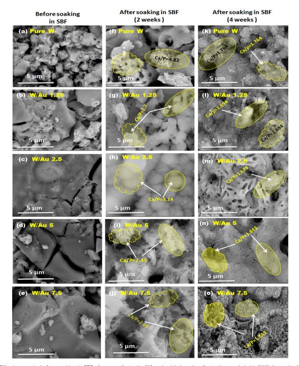
Fig. 4 SEM micrographs before soaking in SBF of pure wollastonite (W) and gold-doped wollastonite nanohybrids (W/Au) samples (treated at 1200  $^{\circ}$ C per 2 h) (a-e) and after immersion in SBF for 2 weeks (f-j) and for 1 month (k-o).
