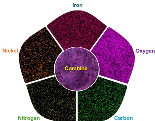
Fig. 5 EDX elemental mapping images of  $[\text{Fe}_3\text{O}_4@\text{salicylamide-L-proline-Ni(II)}]$  nanocomposite.
