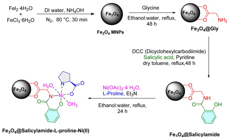
Scheme 1 Stepwise synthesis of  $[\text{Fe}_3\text{O}_4@\text{salicylamide-L-proline-Ni(II)}]$  nanocomposite.
