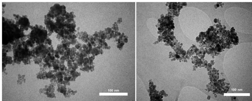
Fig. 7 TEM images of  $[\text{Fe}_3\text{O}_4@\text{salicylamide-L-proline-Ni(II)}]$  nanocomposite.
