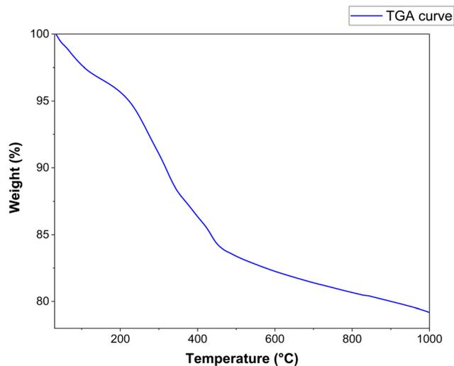
Fig. 3 TGA analysis of  $[\text{Fe}_3\text{O}_4@\text{salicylamide-}L\text{-proline-Ni(II)}]$  nanocomposite.
