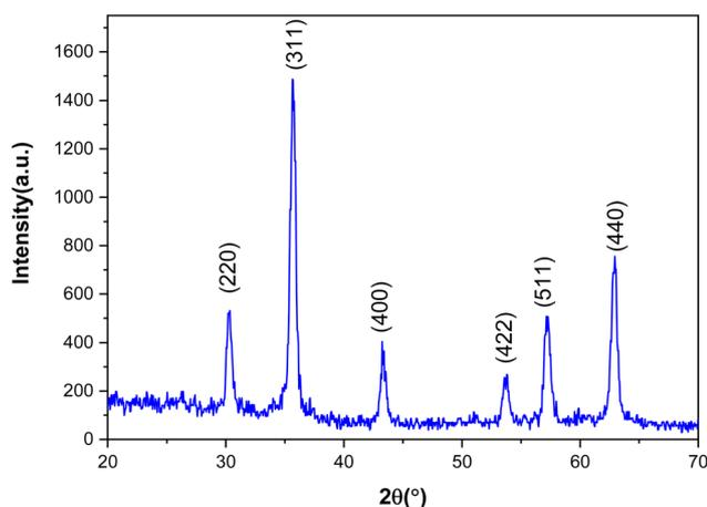
Fig. 2 XRD analysis of  $[\text{Fe}_3\text{O}_4@\text{salicylamide-}L\text{-proline-Ni(II)}]$  nanocomposite.
