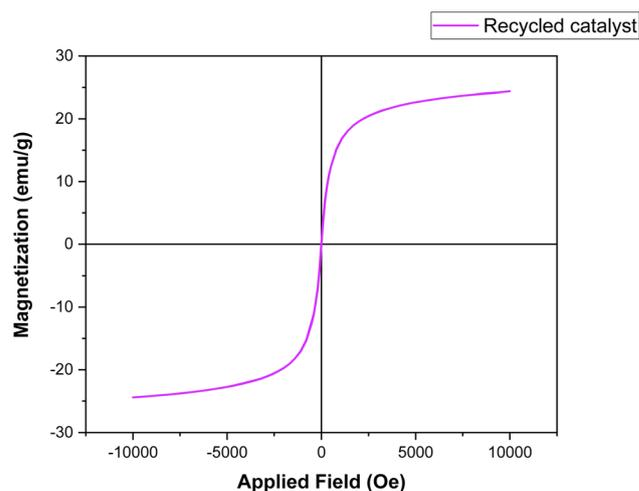
Fig. 12 VSM analysis of recovered  $[\text{Fe}_3\text{O}_4@\text{salicylamide-L-proline-Ni(II)}]$  nanocomposite.
