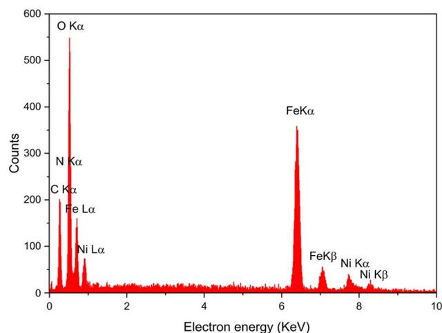
Fig. 4 EDAX analysis of  $[\text{Fe}_3\text{O}_4@\text{salicylamide-}L\text{-proline-Ni(II)}]$  nanocomposite.
