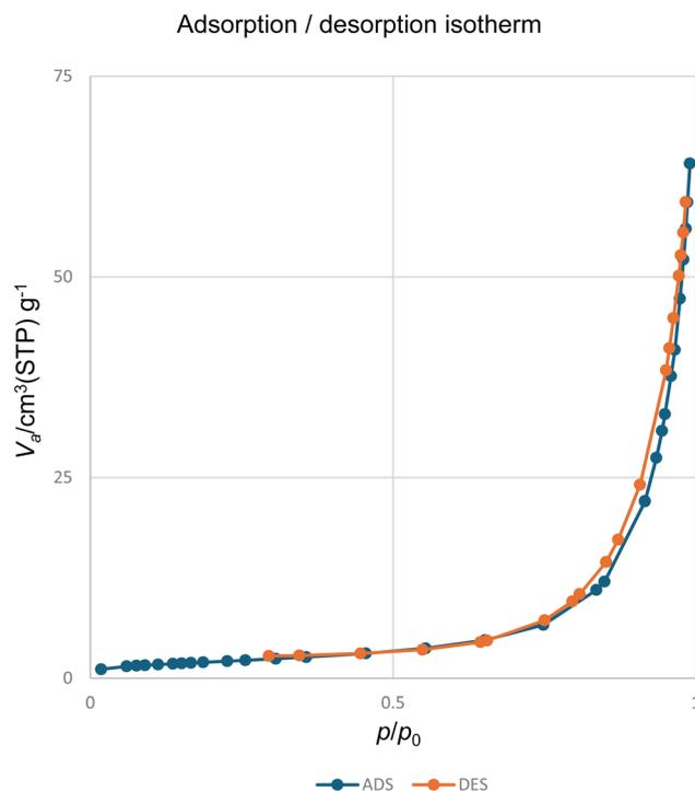
Fig. 9  $\text{N}_2$  adsorption–desorption isotherm of  $[\text{Fe}_3\text{O}_4@\text{salicylamide-L-proline-Ni(II)}]$  nanocomposite.
