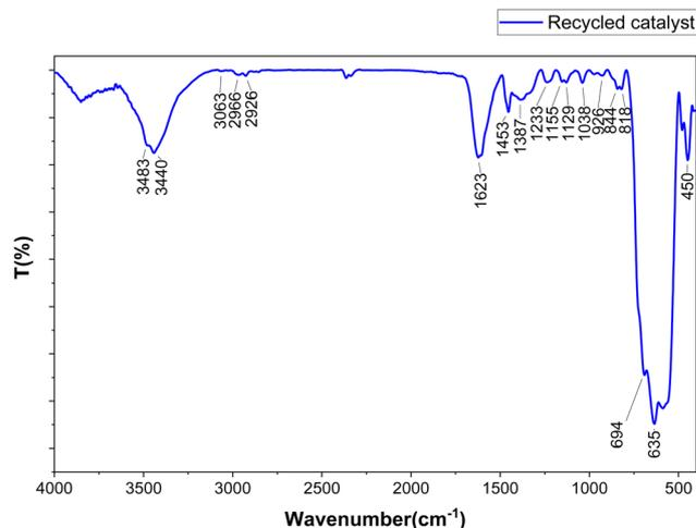
Fig. 11 FT-IR analysis of recovered  $[\text{Fe}_3\text{O}_4@\text{salicylamide-L-proline-Ni(II)}]$  nanocomposite.
