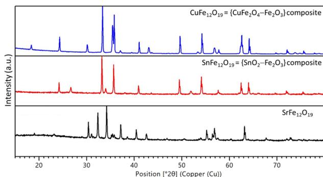
Fig. 1 XRD patterns of  $\text{CuFe}_{12}\text{O}_{19}$ ,  $\text{SnFe}_{12}\text{O}_{19}$  and  $\text{SrFe}_{12}\text{O}_{19}$ .
