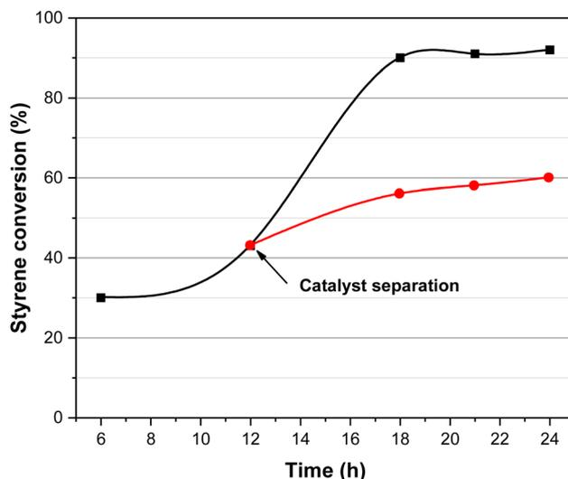
Fig. 11 Heterogeneity test of the CuFe<sub>12</sub>O<sub>19</sub> nanoparticles.
