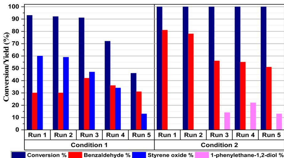
Fig. 12 CuFe<sub>12</sub>O<sub>19</sub> reusability in the gram-scale selective catalytic oxidation of styrene.
