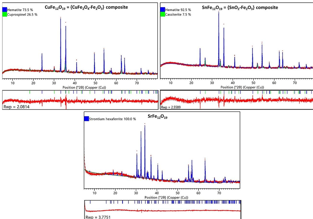
Fig. 2 Rietveld refinement of  $\text{CuFe}_{12}\text{O}_{19}$ ,  $\text{SnFe}_{12}\text{O}_{19}$  and  $\text{SrFe}_{12}\text{O}_{19}$ .
