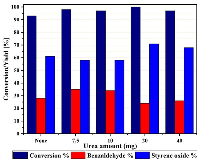
Fig. 10 Effect of urea in the presence of *t*BHP and CuFe<sub>12</sub>O<sub>19</sub> as the catalyst.
