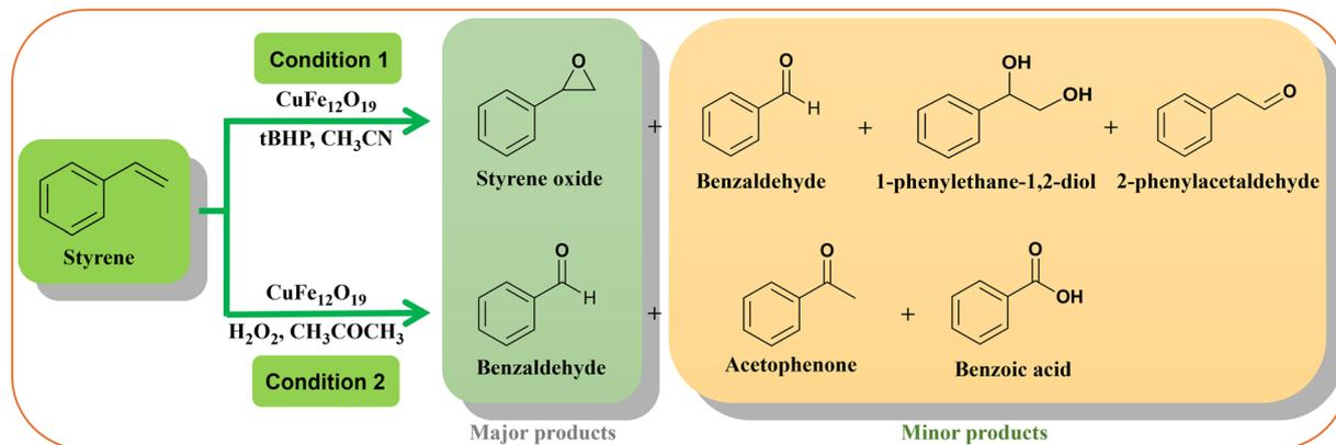
Scheme 2 Catalytic oxidation of styrene in the presence of *t*BHP or H<sub>2</sub>O<sub>2</sub>.Table 4 Comparison of the catalytic activity of the as-prepared nanomaterials in catalytic styrene oxidation<sup>a</sup>
