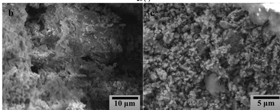
Fig. 13 XRD patterns of the fresh and recycled CuFe<sub>12</sub>O<sub>19</sub> (a), and SEM images of CuFe<sub>12</sub>O<sub>19</sub> after five runs while using (b) tBHP or (c) H<sub>2</sub>O<sub>2</sub>.
