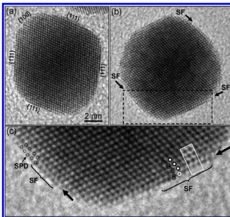
Fig. 8 HRTEM images of (a) Au seed; (b) alloyed bimetallic nanoparticle with single atomic layer of Pd; and (c) magnified HRTEM image from the rectangle-enclosed area in (b)<sup>130</sup> (reproduced with permission, ACS Publisher, 2010).
