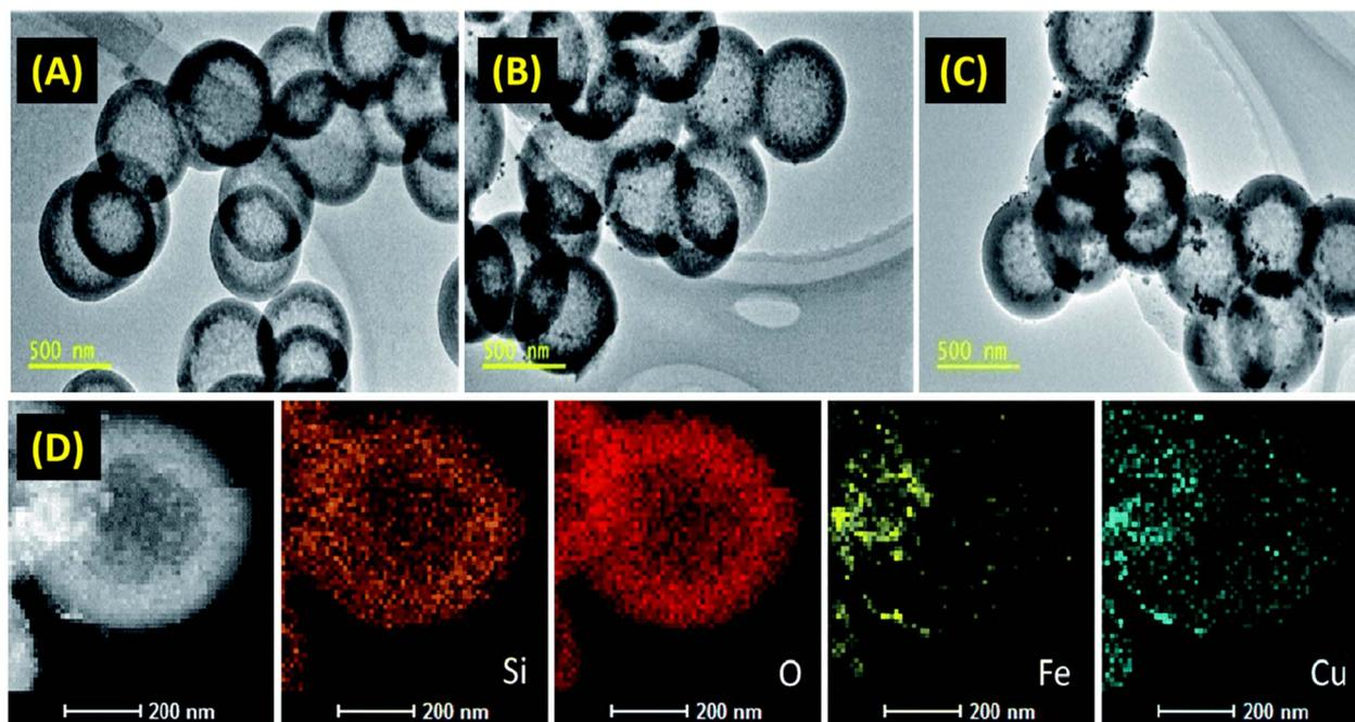
Fig. 5 TEM of (A) blank hollow mesoporous silica sphere; (B) Fe loaded hollow mesoporous silica sphere; (C) Fe–Cu bimetallic hollow mesoporous silica sphere; (D) STEM and elemental mapping images of Fe–Cu bimetallic hollow mesoporous silica sphere<sup>127</sup> (reproduced with permission, RSC Publishing, 2016).
