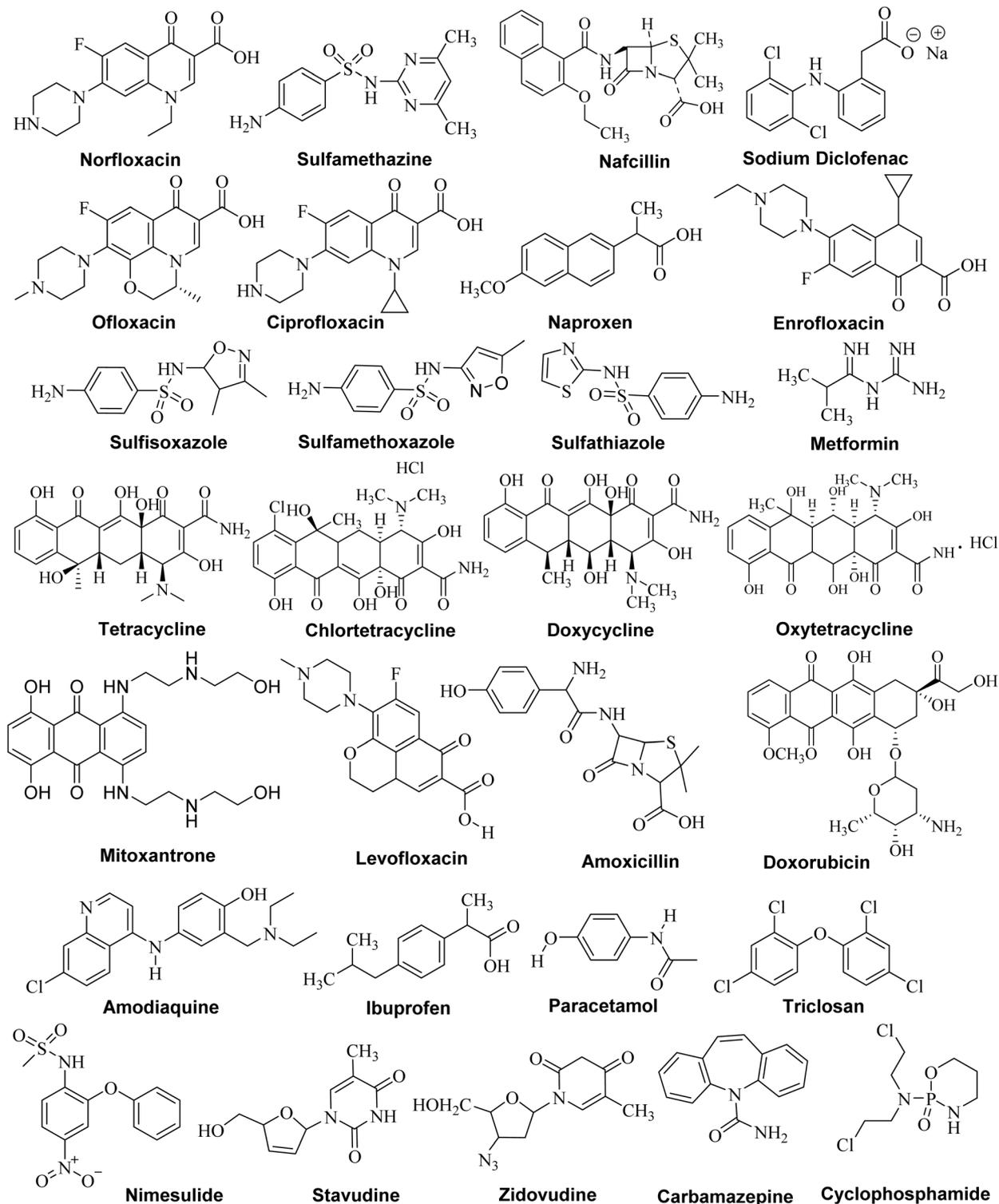
Fig. 11 Structure of various pharmaceuticals used as PPCPs.
