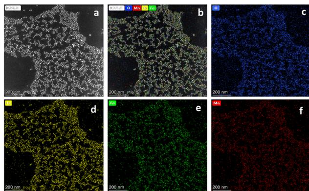
Fig. 5 EDS colour mapping of the  $\text{CoMnFe}_2\text{O}_4$  nanoparticles. (a) HAADF, (b) overlapped, (c) O, (d) Fe, (e) Co and (f) Mn.
