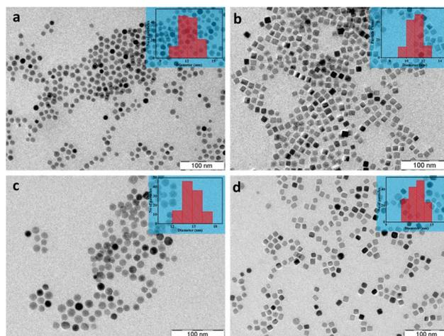
Fig. 4 TEM images of  $MnFe_2O_4$  (a) nanospheres and (b) nanocuboids. TEM images of  $CoMnFe_2O_4$  (c) nanospheres and (d) nanocuboids. The inset shows the particle size histogram.
