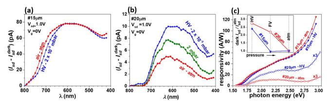
Fig. 4 Spectral photocurrent measured for  $V_g = 0$  on samples #15  $\mu$ m (a) and #20  $\mu$ m (b) at room temperature under vacuum and at different pressures; and (c) comparison of the spectral photoresponsivity computed based on the data in panels (a) and (b) and the calibrated spectral illumination power (the inset shows the dark current  $I_{sd}$  normalized to its value at atmospheric  $I_{sd}^{atm}$ ).
