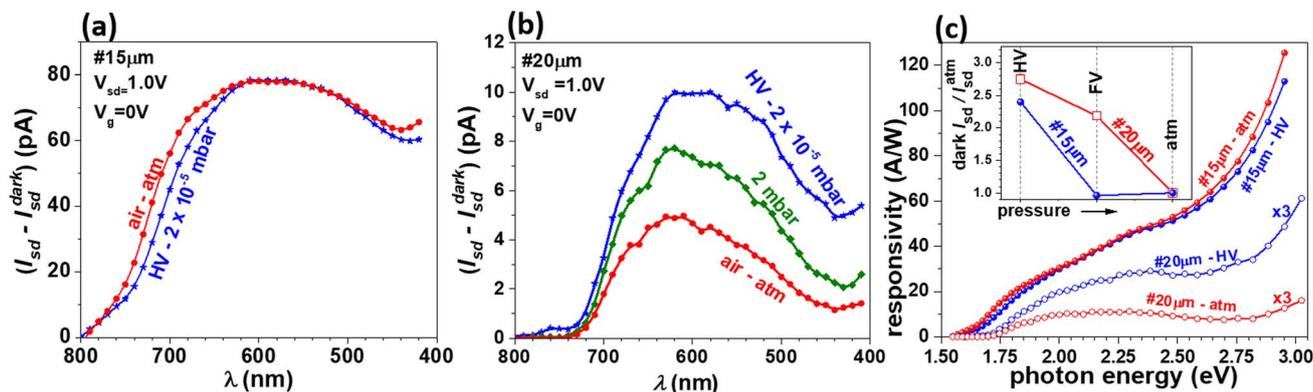
Fig. 4 Spectral photocurrent measured for  $V_g = 0$  on samples #15  $\mu\text{m}$  (a) and #20  $\mu\text{m}$  (b) at room temperature under vacuum and at different pressures; and (c) comparison of the spectral photoresponsivity computed based on the data in panels (a) and (b) and the calibrated spectral illumination power (the inset shows the dark current  $I_{sd}$  normalized to its value at atmospheric  $I_{sd}^{\text{atm}}$ ).
