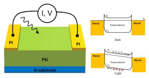
Energy bandgap diagram of the Pt/PSi/Pt device.
