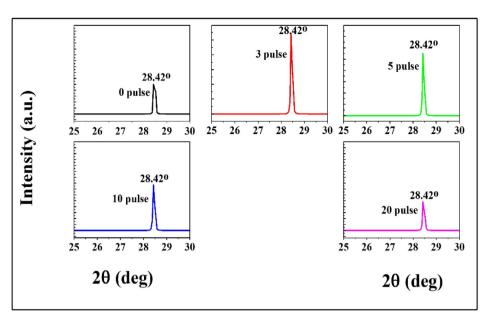
Fig. 5 XRD patterns of the n-PSi samples annealed under varying laser pulses.
