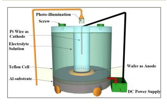
Fig. 1 Graphical representation of the PECE cell used to generate n-PSi samples.
