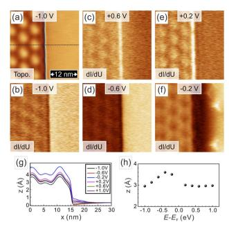
Fig. 4 (a) Zoom-in topography at the edge proximity of  $\alpha$ -FeTe/ Bi<sub>2</sub>Te<sub>3</sub>. The surface morphology of the moiré superlattice stays the same within the bias voltage range of  $\pm 1.0$  eV. (b)–(f) Bias-dependent conductance maps reveal the local intensity of tunneling conductance spatially modulated within the moiré superlattice. (g) Bias-dependent height profiles along the black dashed line in (a) and an apparent height of 3.2 Å on average can be extracted from (h).
