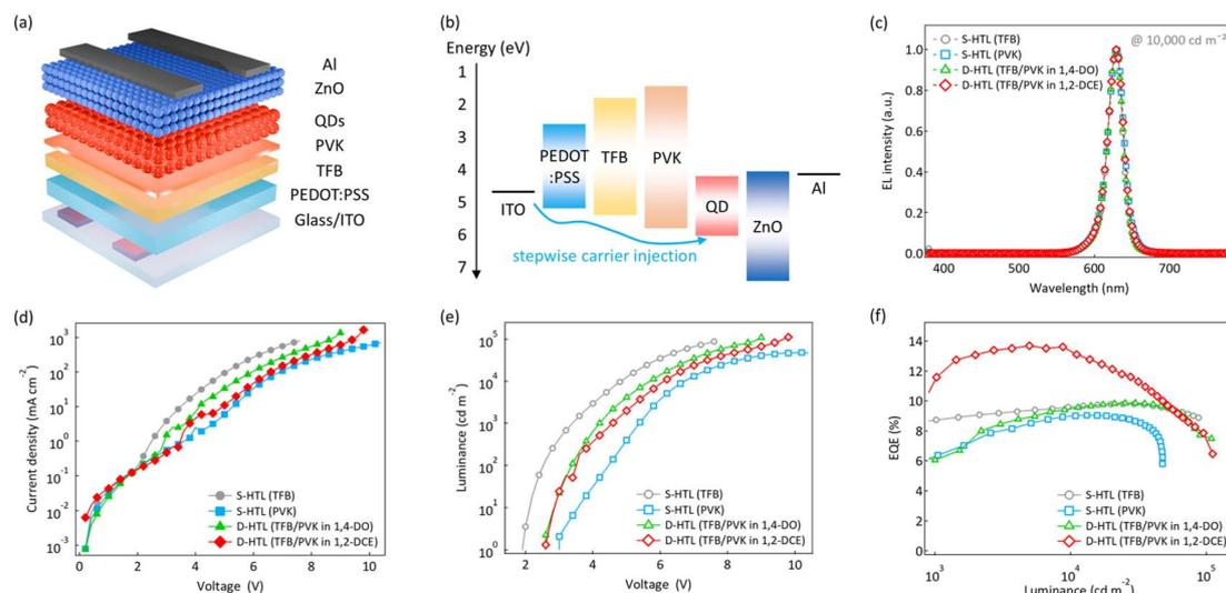
Fig. 4 Schematic illustration of (a) the device structure and (b) the energy band diagram for QD-LEDs incorporating TFB/PVK D-HTLs. (c–f) The performance of QD-LEDs using TFB/PVK D-HTLs processed with either 1,2-DCE and 1,4-DO, compared with the devices featuring an S-HTL (TFB or PVK): (c) normalized EL spectrum, (d) current density–voltage characteristics, (e) luminance–voltage characteristics, and (f) external quantum efficiency–luminance characteristics.
