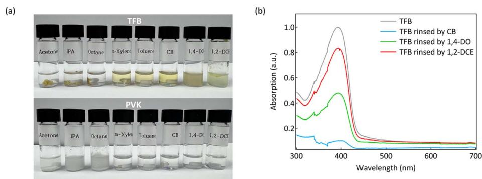
Fig. 1 (a) Photographs of TFB and PVK in different solvents. The solvents from left to right are acetone, IPA, octane, *m*-xylene, toluene, chlorobenzene (CB), 1,4-dioxane (1,4-DO), and 1,2-dichloroethane (1,2-DCE). (b) Absorption spectra of TFB films with and without rinsing with different solvents.
