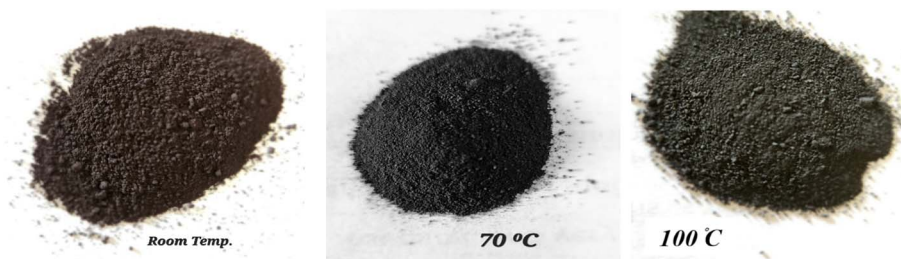
Fig. 3 Photographs of NbSe 2 nanoparticles synthesized at different temperatures.
