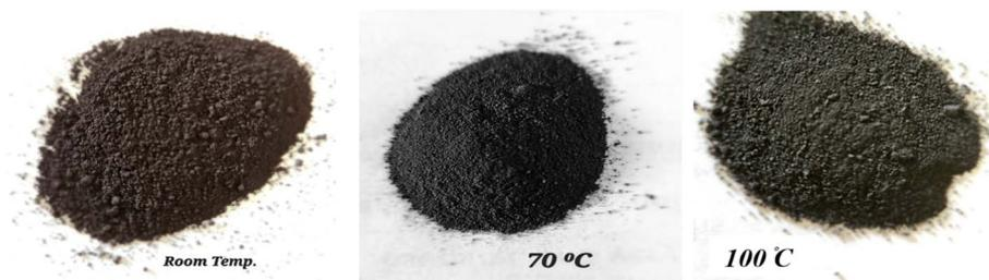
Fig. 3 Photographs of NbSe<sub>2</sub> nanoparticles synthesized at different temperatures.
