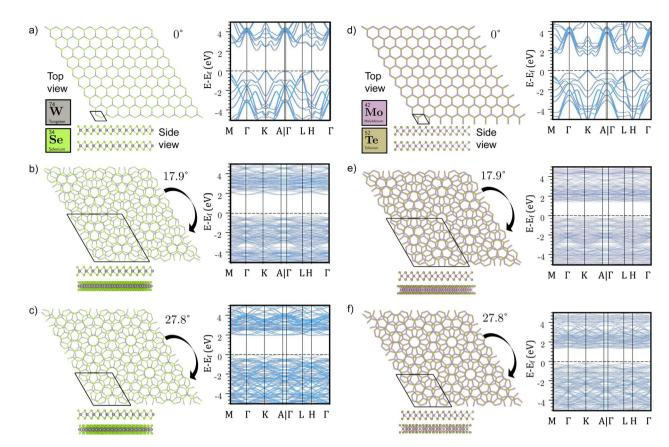
Fig. 4 Geometries and band structures of bilayer WSe<sub>2</sub> at various twisted angles are shown for (a)  $0^{\circ}$ , (b)  $17.9^{\circ}$ , (c)  $27.8^{\circ}$ as well as MoTe<sub>2</sub> (d-f) for the corresponding angles. Each panel provides both a top view and a side view of the bilayer geometries (shown in the bottom left of each section). For a broader perspective, analogous analyses for other materials including  $1H-MoS_2$ ,  $1T-MoS_2$
