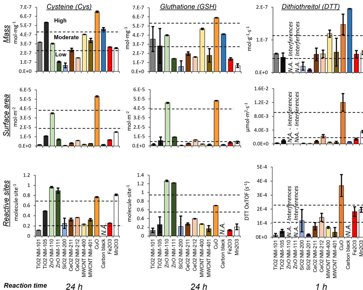
Fig. 2 Oxidative potential of the tested ENMs evaluated based on Cys (left) and GSH (center) 24 h consumption and the DTT 1 h oxidation rate (right) normalized by mass (top), surface area (middle) and reactive site (bottom). Averaged values ( $n = 3$ ) with error bars indicating the standard deviation. Statistical clustering by the  $k$ -means algorithm according to reactivity (high-moderate-low) is indicated by horizontal dashed lines.
