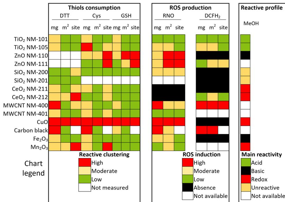
Fig. 4 Heat map for the 14 ENMs evaluated based on their intrinsic oxidative capacity to react with the thiol group in DTT, Cys, and GSH, or their production of ROS that are trapped by RNO and DCFH<sub>2</sub>, as well as based on their reactive profile obtained via methanol temperature programmed surface reaction. Clustering was performed by the *k*-means algorithm.
