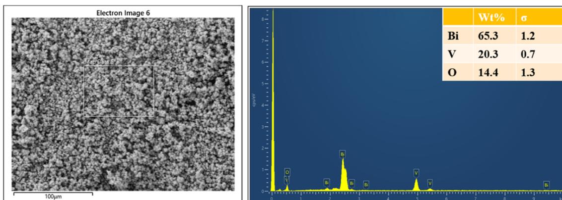
Fig. 3 Energy-dispersive X-ray (EDX) spectrum of the synthesized  $\text{BiVO}_4$  nanospheres.
