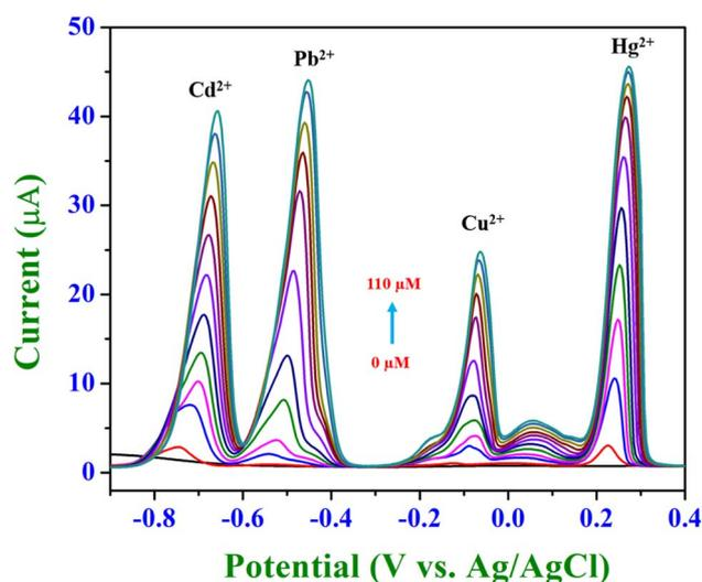
Fig. 10 SWASV voltammograms for the simultaneous detection of  $\text{Cd}^{2+}$ ,  $\text{Pb}^{2+}$ ,  $\text{Cu}^{2+}$  and  $\text{Hg}^{2+}$  using  $\text{BiVO}_4/\text{GCE}$ . Anodic peaks corresponding to each metal are observed in the concentration range of 0–110  $\mu\text{M}$ .
