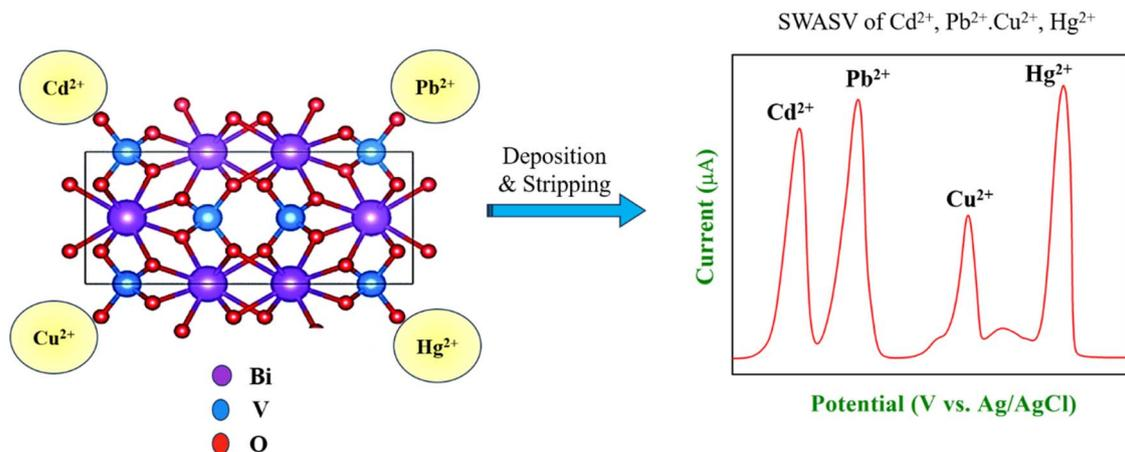
Fig. 8 The graphical illustration of the adsorption mechanism of heavy metal ions on the surface of  $\text{BiVO}_4/\text{GCE}$  in 0.1 M HEPES buffer determined by SWASV.<sup>50</sup>
