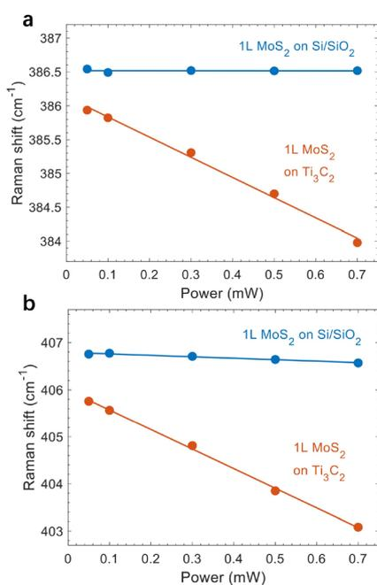
Fig. 5 Raman peak positions as a function of excitation power. (a and b) Peak positions of the E<sub>2g</sub><sup>1</sup> (a) and A<sub>1g</sub> (b) modes. Dots represent experimental data and lines correspond to a linear fitting.
