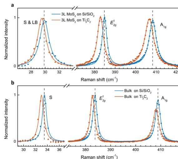
Fig. 4 Raman spectra of 3L (a) and bulk (b) MoS<sub>2</sub> on Ti<sub>3</sub>C<sub>2</sub> MXene in comparison with the counterparts on Si/SiO<sub>2</sub>.
