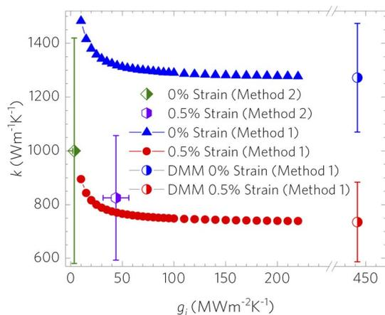
Fig. 7 Relationship between interfacial thermal conductance ( $g_i$ ) and in-plane thermal conductivity ( $k$ ) for monolayer graphene coated onto a Cu substrate. Analysis was performed using both one- and two-objective optothermal Raman thermometry techniques, denoted as methods 1 and 2, respectively.
