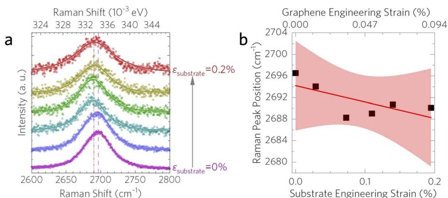
Fig. 3 (a) Raman spectra and (b) peak position showing a red shift of the graphene 2D peak with respect to substrate engineering tensile strain excited at  $P = 2.9$  mW. The shaded area in (b) indicates the 99% confidence interval band of a linear fit to the data.
