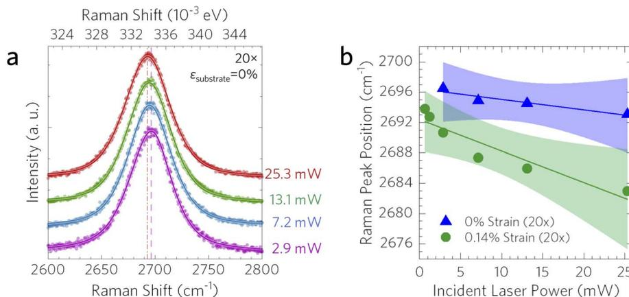
Fig. 5 Power dependent Raman spectra for graphene on copper (method 1). (a) Incident laser power dependent ( $P = 2.9$ – $25.3$  mW) Raman spectra for unstrained graphene on copper, and (b) 2D peak position for 0% and 0.14% substrate engineering strain. Linear fits to the data are shown along with the 99% confidence interval bands.
