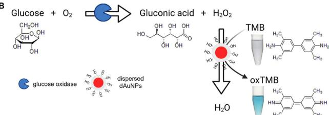
Fig. 3 Schematic mechanism for the dual-functional tablet sensor. (A) The tablet acts as a plasmonic sensor detecting uric acid; (B) the tablet acts as a nanozyme sensor detecting glucose.
