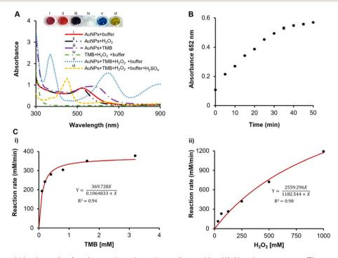
Fig. 6 Optimization and kinetic studies for glucose detection using a direct tablet. (A) Absorbance spectra; (B) a graph showing a gradual increase in the concentration of oxTMB with time; (C) steady-state kinetics of a dAuNP tablet.
