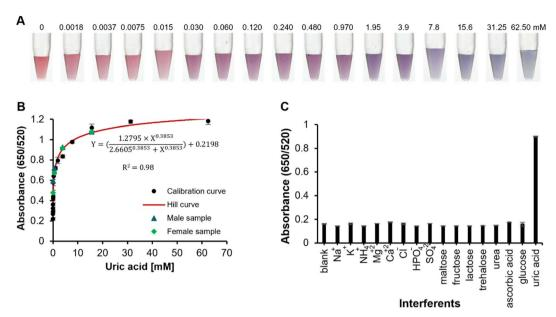
Fig. 5 Detection of uric acid using a dual-functional tablet sensor. (A) Optimal images of color transition in a reaction vial; (B) a calibration plot indicating a concentration-dependent response of a direct tablet for uric acid along with real-sample spiking results; (C) selectivity of the proposed dual-functional tablet sensor.
