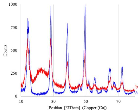
Fig. 7 XRD patterns of (a) boehmite and (b) boehmite@Schiff-base-Cu nanocatalyst.
