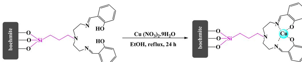
Scheme 5 Synthesis of the boehmite@Schiff-base-Cu nanocatalyst.
