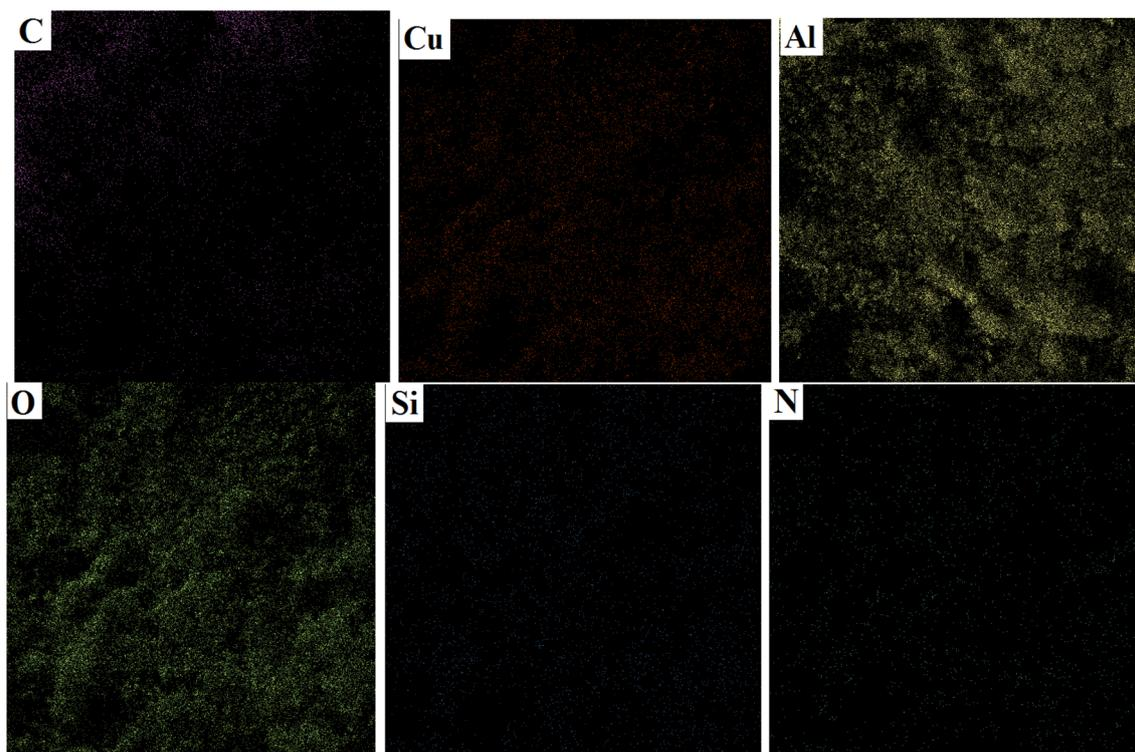
Fig. 5 Elemental mapping images of the boehmite@Schiff-base-Cu nanocatalyst.
