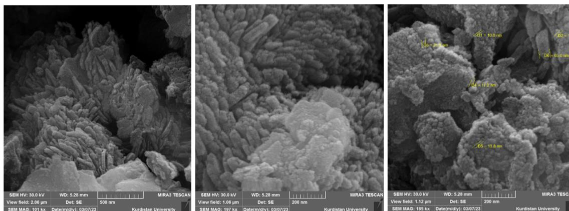
**Fig. 3** SEM images of the boehmite@Schiff-base-Cu nanocatalyst.
