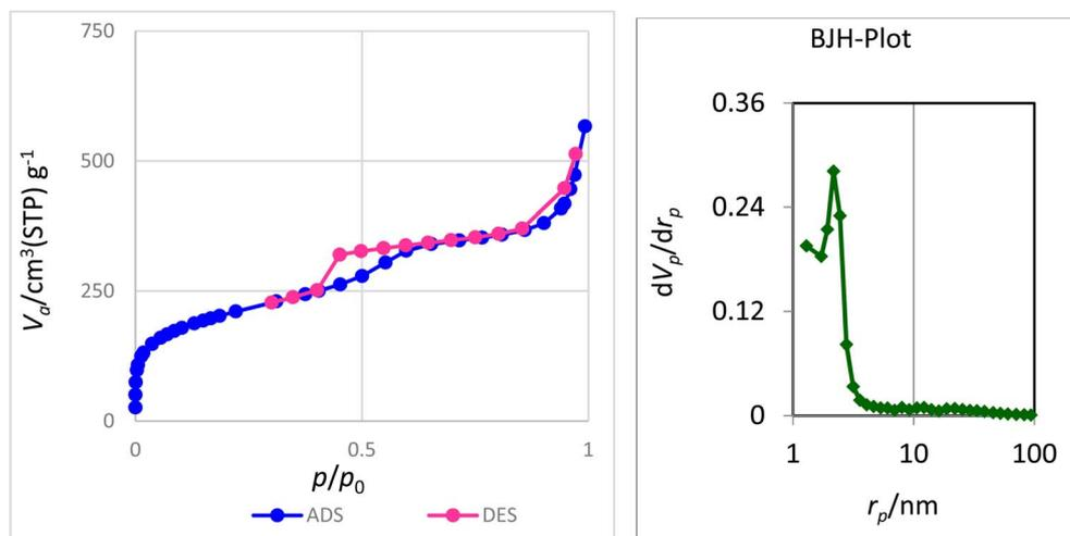
Fig. 1  $\text{N}_2$  adsorption–desorption isotherms and BJH-plot of the boehmite@Schiff-base-Cu nanocatalyst.
