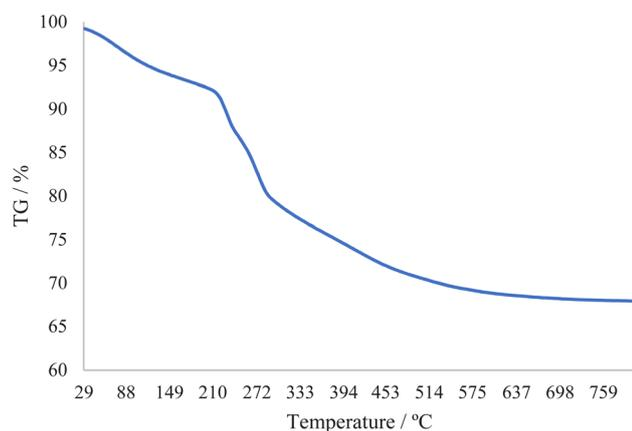
**Fig. 2** TGA curves of the boehmite@Schiff-base-Cu nanocatalyst.
