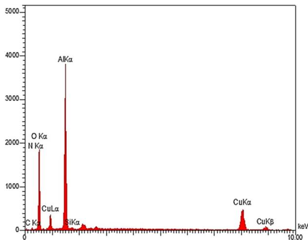
Fig. 4 The EDS spectra of the boehmite@Schiff-base-Cu nanocatalyst.
