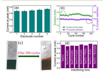
Fig. 5 (a) Reproducibility, (b) reusability of the HPHM electrode, (c) photographs of the electrode before and after the experiment, and (d) DPV response of 10 ppb Se(IV) ions in the presence of various interfering ions (100 ppb).
