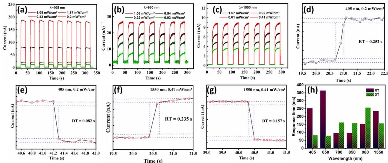
Fig. 4 The dynamic photoresponse characteristic curve of the PVPD at different wavelengths and light power densities (a) 405 nm, (b) 980 nm, and (c) 1550 nm; enlarged portion of the  $I-t$  curve edge on rise (RT) and decay time (DT) of PVPD under (d and e) 405 nm and (f and g) 1550 nm illumination; (h) graphical chart for the response time at different wavelengths.
