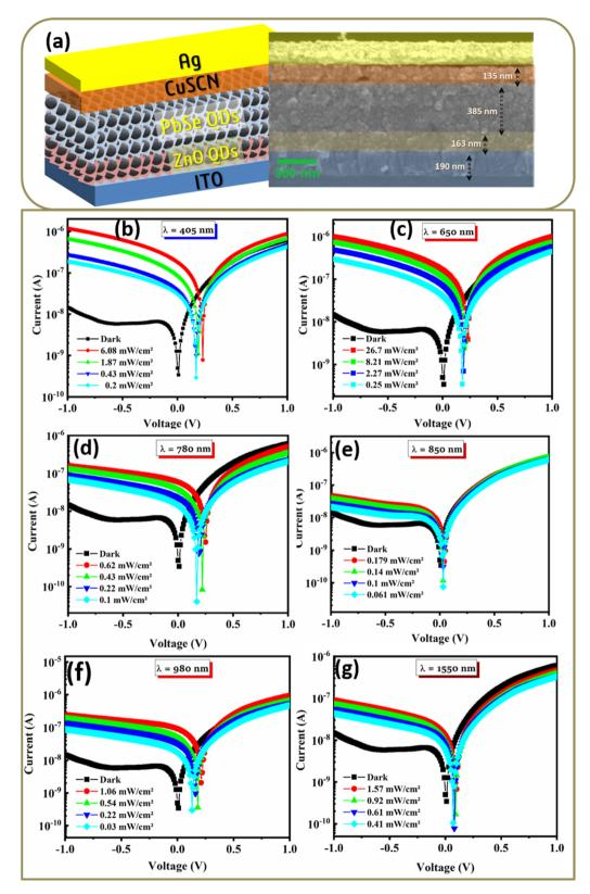
Fig. 2 (a) Schematic illustration of the photovoltaic PD (left side) and cross-sectional FESEM image of the PD with device structure ITO/ZnO (163 nm)/PbSe QDs (385 nm)/CuSCN (135 nm)/Ag (right side); I-V plot of the PD at various optical power densities under (b) 405 nm, (c) 650 nm, (d) 780 nm, (e) 850 nm, (f) 980 nm and (g) 1550 nm illumination.
