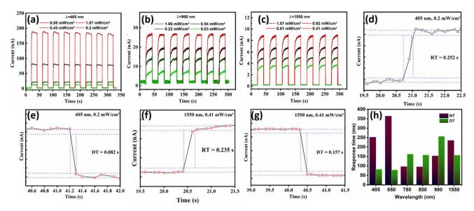
Fig. 4 The dynamic photoresponse characteristic curve of the PVPD at different wavelengths and light power densities (a) 405 nm, (b) 980 nm, and (c) 1550 nm; enlarged portion of the I-t curve edge on rise (RT) and decay time (DT) of PVPD under (d and e) 405 nm and (f and g) 1550 nm illumination; (h) graphical chart for the response time at different wavelengths.
