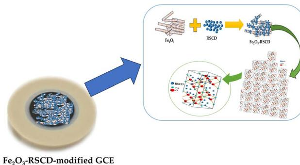
Scheme 2 Fabrication of Fe<sub>2</sub>O<sub>3</sub>-RSCD-modified GCE for electrochemical analysis.
