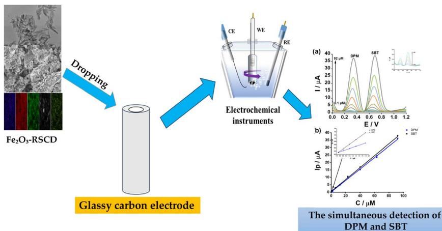
Scheme 3 Flow chart of preparing  $\text{Fe}_2\text{O}_3\text{-RSCD/GCE}$ .
