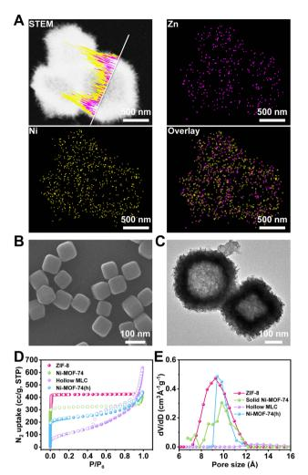
Fig. 2 (A) STEM, EDS elemental mapping images and line scan patterns of the hollow MLC. (B) SEM image of cubic ZIF-8. (C) TEM images of the hollow MLC with a cubic cavity. (D) N2 adsorptiondesorption isotherms at 77 K of ZIF-8, solid Ni-MOF-74, the hollow MLC and solid Ni-MOF-74(h). (E) Pore size distribution of ZIF-8, solid Ni-MOF-74, the hollow MLC and Ni-MOF-74(h).
