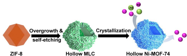
Scheme 1 Hollow Ni-MOF-74 was synthesized by a two-step process to enhance the dynamic separation of Xe/Kr.
