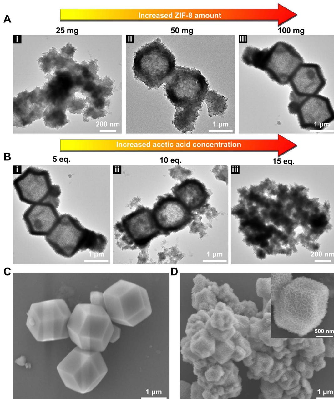
**Fig. 1** (A) TEM images of the hollow MLC synthesized with various amounts of ZIF-8. (B) TEM images of the hollow MLC synthesized with various amounts of HOAc. SEM images of dodecahedral ZIF-8 (C) and the hollow MLC (D).
