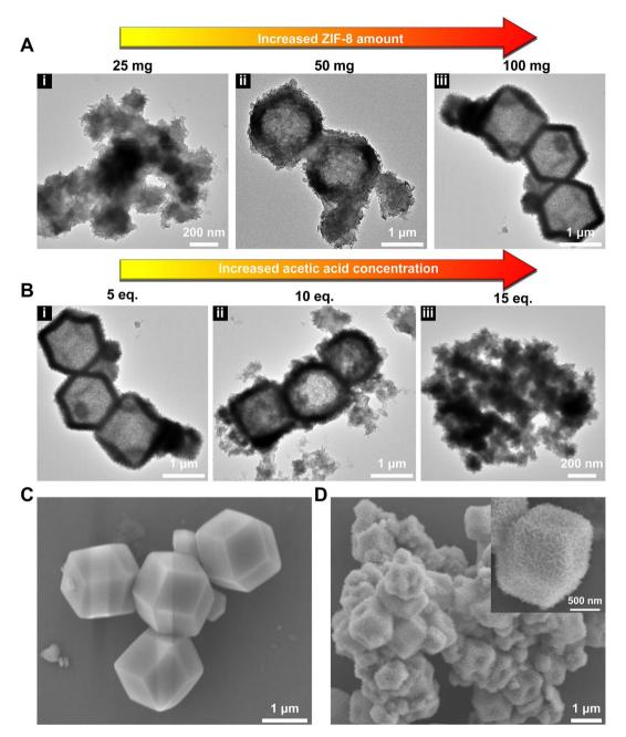
Fig. 1 (A) TEM images of the hollow MLC synthesized with various amounts of ZIF-8. (B) TEM images of the hollow MLC synthesized with various amounts of HOAc. SEM images of dodecahedral ZIF-8 (C) and the hollow MLC (D).
