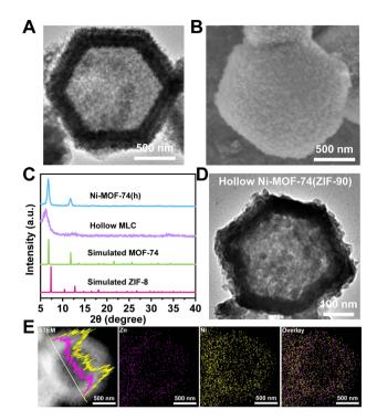
Fig. 3 SEM (A) and TEM (B) images of Ni-MOF-74(h). (C) PXRD patterns of the hollow MLC and Ni-MOF-74(h). (D) TEM image of Ni-MOF-74(h) by using ZIF-90 as the template. (E) STEM, EDS elemental mapping images and line scan patterns of Ni-MOF-74(h).
