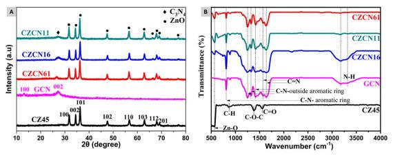
Fig. 1 (A) Diffractograms and (B) FTIR spectra of the synthesized CZ45, GCN, and CZCN samples.
