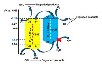
Fig. 12 A plausible OFL photodegradation mechanism on the CZCN11 composite.
