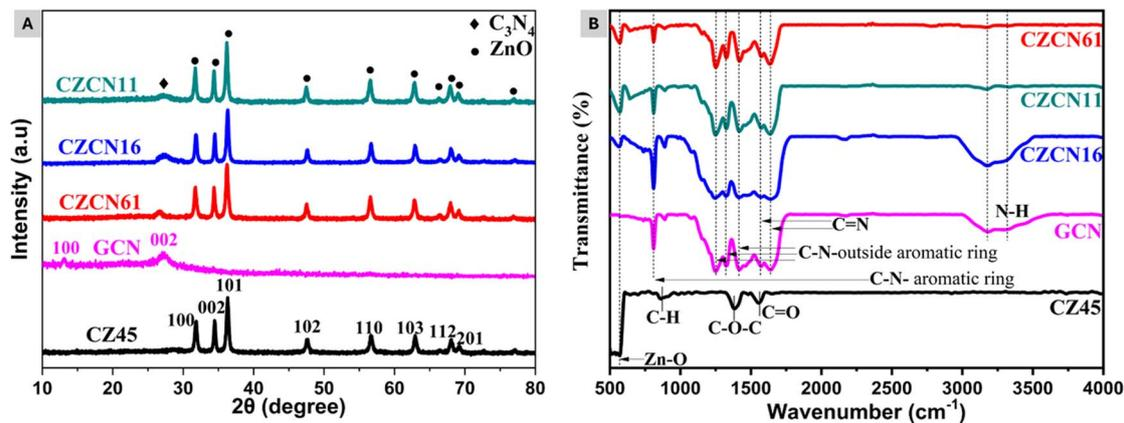
Fig. 1 (A) Diffractograms and (B) FTIR spectra of the synthesized CZ45, GCN, and CZCN samples.
