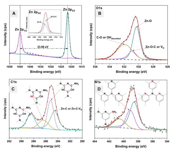
Fig. 4 High-resolution XPS spectra of the (A) Zn 2p (inset figure: the deconvolution of Zn 2p<sub>3/2</sub> peak), (B) O 1s, (C) C 1s, and (D) N 1s core levels of the CZCN11 composite (black dashed line: raw data, blue dashed line: baseline, red line: fitting line, other lines: deconvoluted lines).
