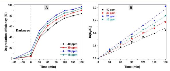
Fig. 8 Influence of the initial OFL concentration on the (A) degradation efficiency and (B) degradation rate of OFL.
