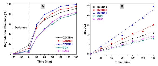
Fig. 6 (A) Efficiency and (B) fitted first-order kinetic model for the photodegradation of OFL by the prepared materials.
