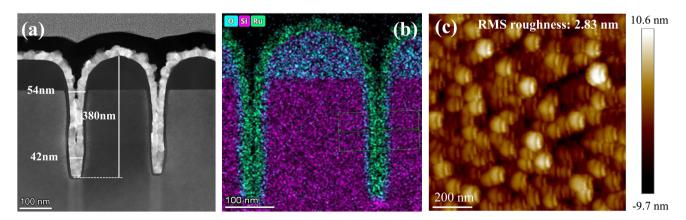
Fig. 4 ALD Ru films for filling the nanoTSV arrays under the condition of deposition temperature of 300 °C, Ru(EtCp)<sub>2</sub> pulse time for 3 s and the pulse time of  $O_2$  was fixed to 12 s. (a) TEM image of Ru filling for nanoTSV. (b) TEM elemental analysis. (c) AFM image (1 × 1  $\mu$ m) of Ru film surface.
