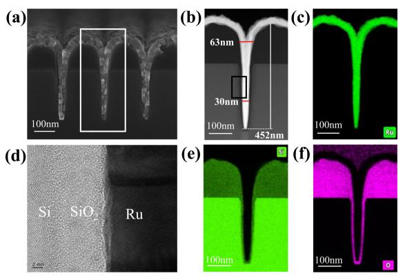
Fig. 7 ALD Ru films for filling the nanoTSV arrays at a temperature of 275 °C, Ru(EtCp)<sub>2</sub> pulse time of 2 s and  $O_2$  exposure time of 12 s. (a) Sideview SEM images of nanoTSV filled with Ru. (b) Side-view TEM images of nanoTSV filled with Ru. (c) Elemental analysis of Ru via TEM. (d) Lattice analysis via TEM. (e) Elemental analysis of Si via TEM. (f) Elemental analysis of O via TEM.
