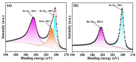
Fig. 3 XPS of ALD Ru films deposited on  $SiO_2/Si$  substrates at temperatures of 300 °C: (a) the  $Ru(EtCp)_2$  pulse time for 1 s. (b) The  $Ru(EtCp)_2$  pulse time for 3 s.
