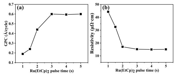
Fig. 2 ALD Ru films deposited on  $SiO_2/Si$  substrates at 300 °C as a function of Ru(EtCp)<sub>2</sub> pulse time. The pulse time of  $O_2$  was fixed to 12 s and the number of ALD deposition cycles was 750: (a) the dependence of GPC on Ru(EtCp)<sub>2</sub> pulse time. (b) The dependence of resistivity on Ru(EtCp)<sub>2</sub> pulse time.
