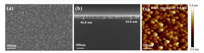
Fig. 6 Plan-view (a) and side-view (b) scanning electron microscopy (SEM) images of Ru films deposited on 10 nm SiO<sub>2</sub>/Si substrates at 275 °C after 750 ALD cycles with an Ru(EtCp)<sub>2</sub> pulsing time of 2 s and O<sub>2</sub> exposure time of 12 s. (c) AFM image  $(1 \times 1 \mu m)$  of the Ru film surface.
