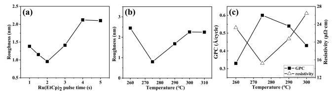
Fig. 5 (a) The dependence of roughness on the Ru(EtCp)<sub>2</sub> pulse time. (b) The dependence of roughness on the deposition temperature. (c) The dependence of GPC and resistivity of ALD Ru films on temperature. The pulse time of O2 was fixed at 12 s and the number of deposition cycles was 750
