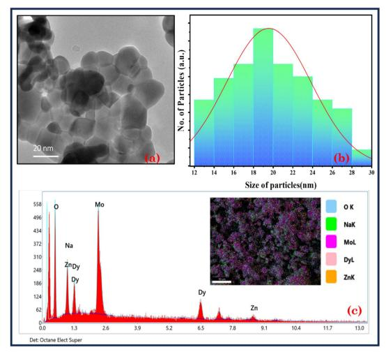
Fig. 4 (a) HR-TEM image of NZMO:6 mol%  $Dy^{3+}$ , (b) particle size histogram of NZMO:6 mol%  $Dy^{3+}$  and (c) EDX spectra of NZMO:6 mol%  $Dy^{3+}$ ; inset of (c) elemental mapping image of NZMO:6 mol%  $Dy^{3+}$ .
