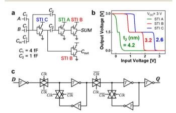
Fig. 4 (a) Circuit diagram of a ternary full adder using capacitors. (b) Simulated transfer characteristics of standard ternary inverters (STIs) A, B, and C. (c) Circuit diagram of the ternary flip-flop. The inverter symbol with a capital "T" represents STI B.
