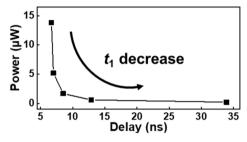
Fig. 6 Simulation result showing the tradeoff relationship between power and delay with a reduction in the first ZnO layer thickness  $t_1$ .
