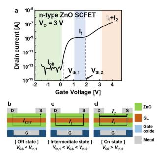
Fig. 2 (a) Experimental  $I_{\rm D}$ – $V_{\rm G}$  characteristics of the n-type ZnO SCFET. The current transport mechanism for ternary operation of n-type SCFETs at (b) off state, (c) intermediate state, and (d) on state.
