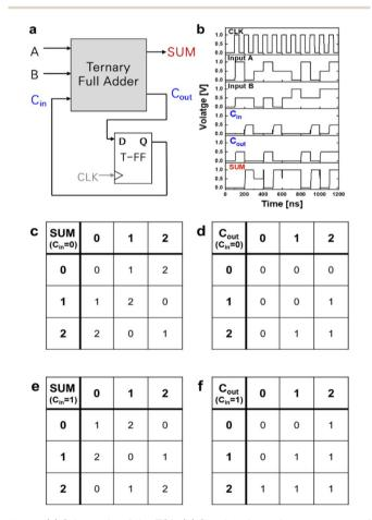
Fig. 5 (a) Schematic of the TSA. (b) Simulated transient responses of the TSA; simulation was performed using Synopsis HSPICE. Truth tables of (c) SUM and (d)  $C_{out}$  when  $C_{in} = 0$  and (e) SUM and (f)  $C_{out}$ when  $C_{in} = 1$ .
